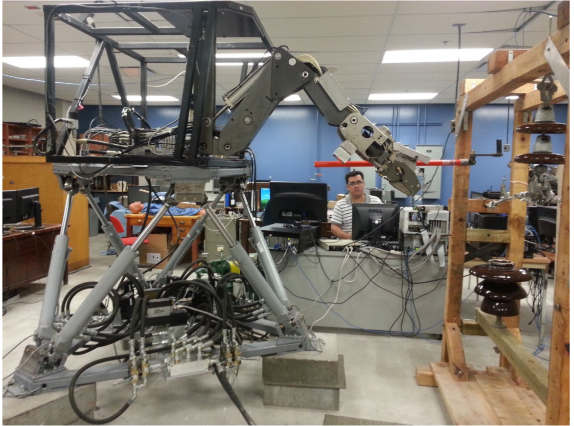
Figure 3.4 Teleoperated hydraulic manipulator setup. The superscript “*” in P_{e,d}^{s*} and F_m^* denotes a delayed/lossy version of displacement and force.
