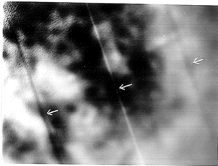
Figure 2.12: The magnetic contrast reverses when the overfocusing changes to underfocusing.
