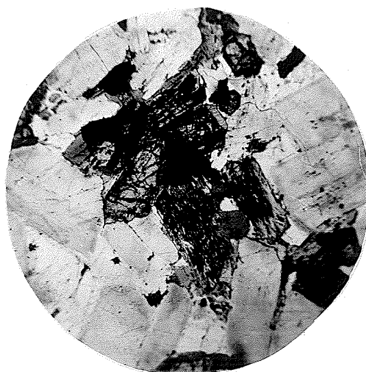
Fig. 3. (xl4) Cluster of hypersthene grains in all stages of alteration.
