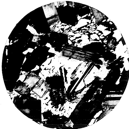
Fig. 2. (xl2) Quartz and granophyre interstitial to feldspar and slightly corroding it. (x-nicols.)
