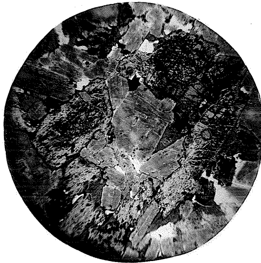
Fig. 4. (x14) Hypersthene almost completely altered to serpentine. Diallage still fresh.
