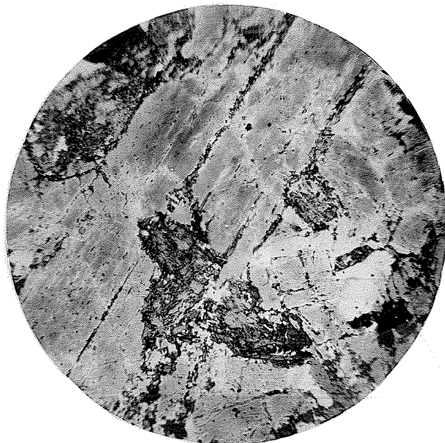
Fig. 6. (xl8) Uralite replacing feldspar along grain boundaries and in irregular patches.
