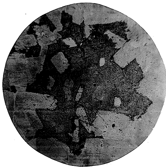
Fig. 1. (xl2) Diplage showing typical irregular shape and enclosing euhedral plagioclase.
