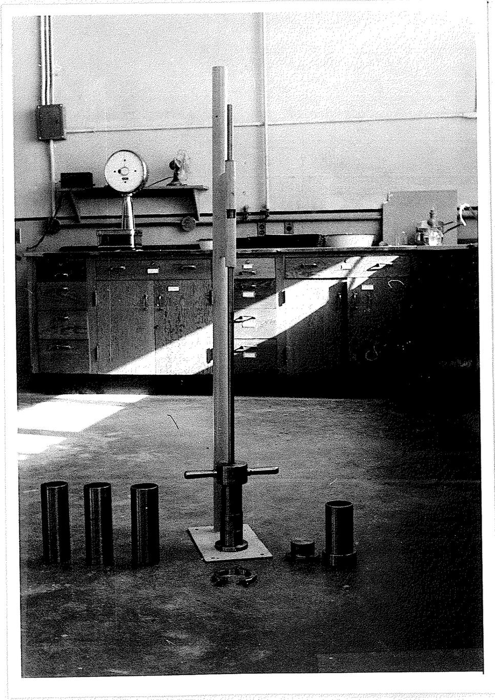
Figure II Specimen Moulding Apparatus
