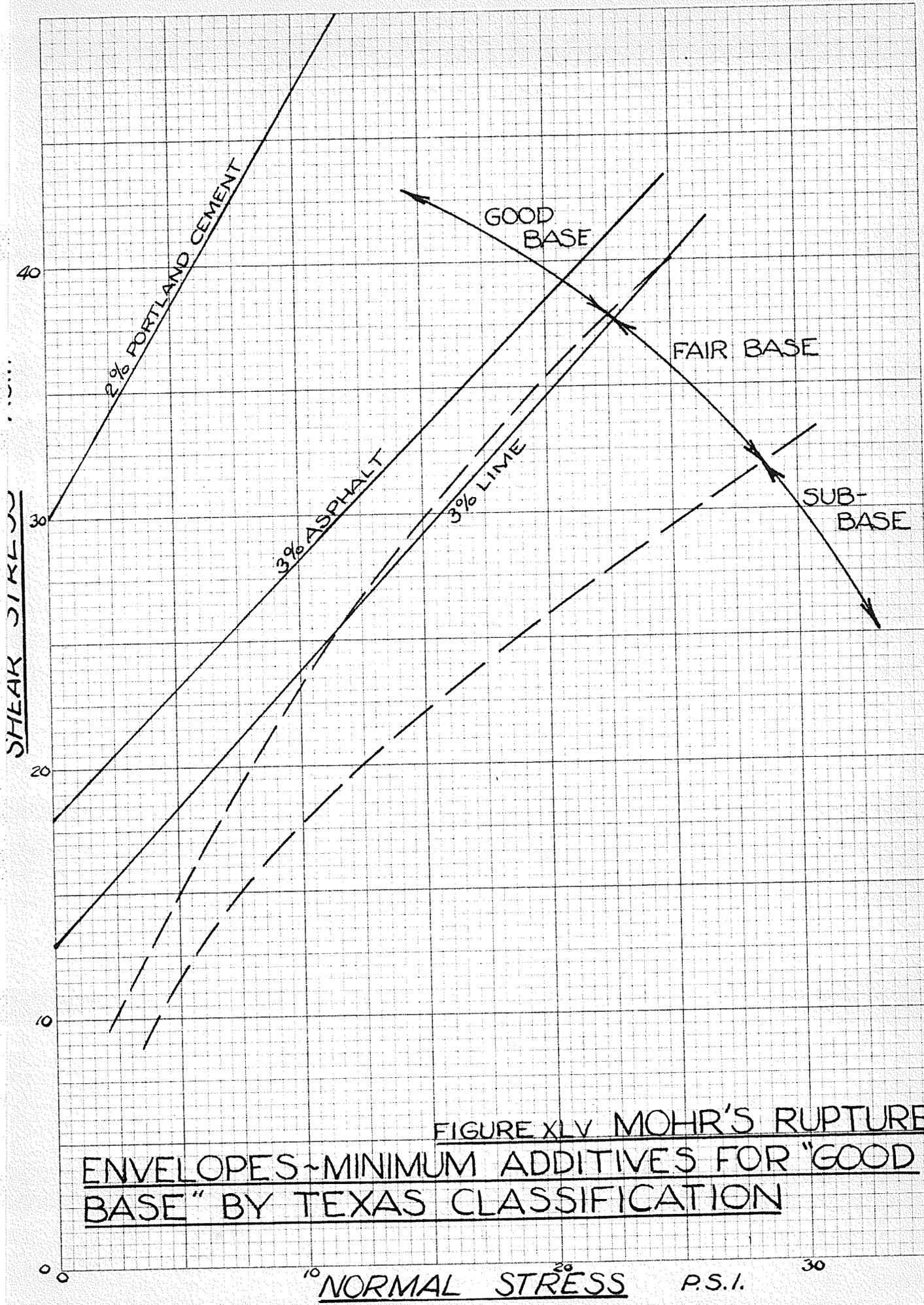
FIGURE XLV MOHR'S RUPTURE ENVELOPES - MINIMUM ADDITIVES FOR "GOOD BASE" BY TEXAS CLASSIFICATION
