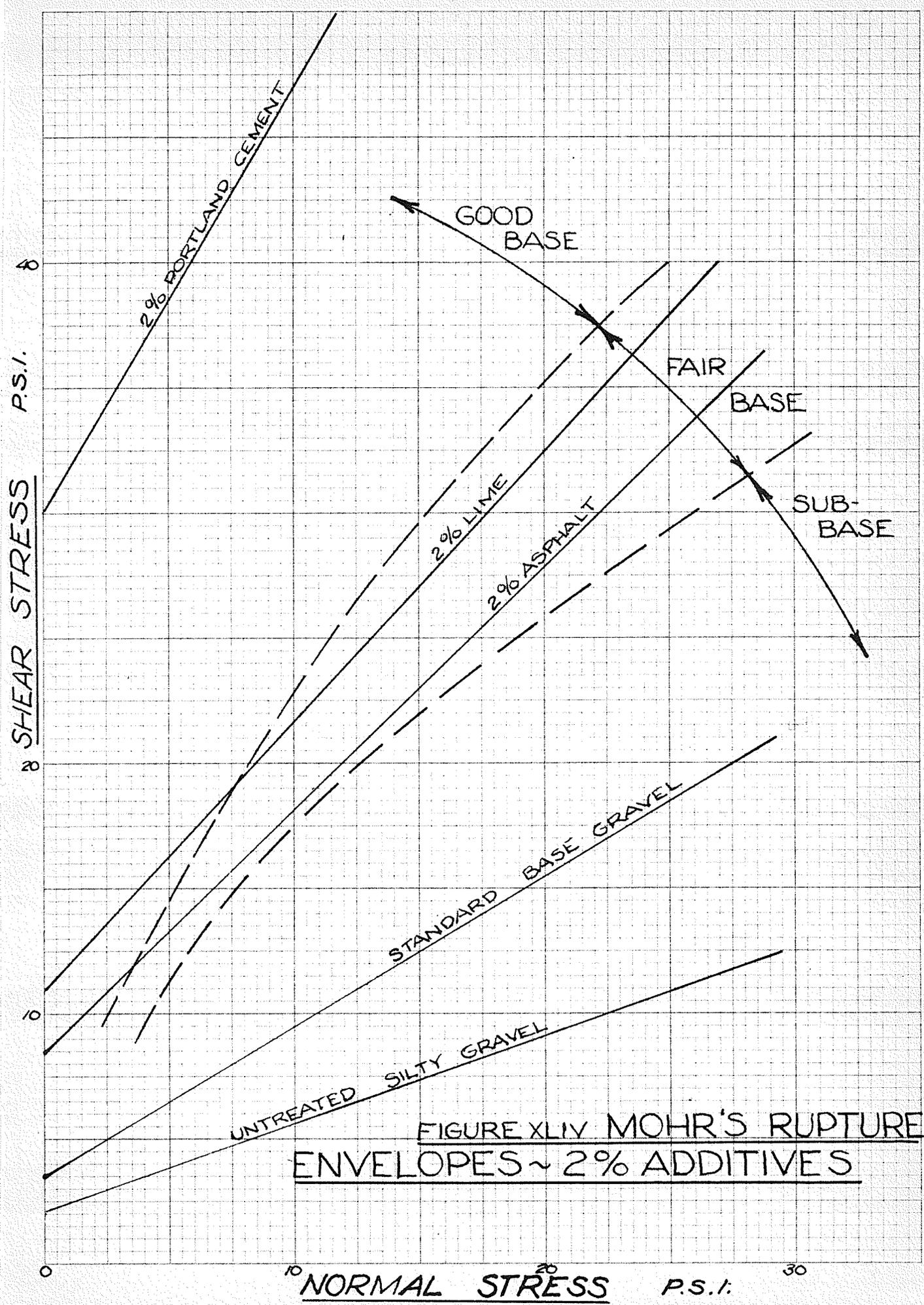
FIGURE XLIV MOHR'S RUPTURE ENVELOPES ~ 2% ADDITIVES
