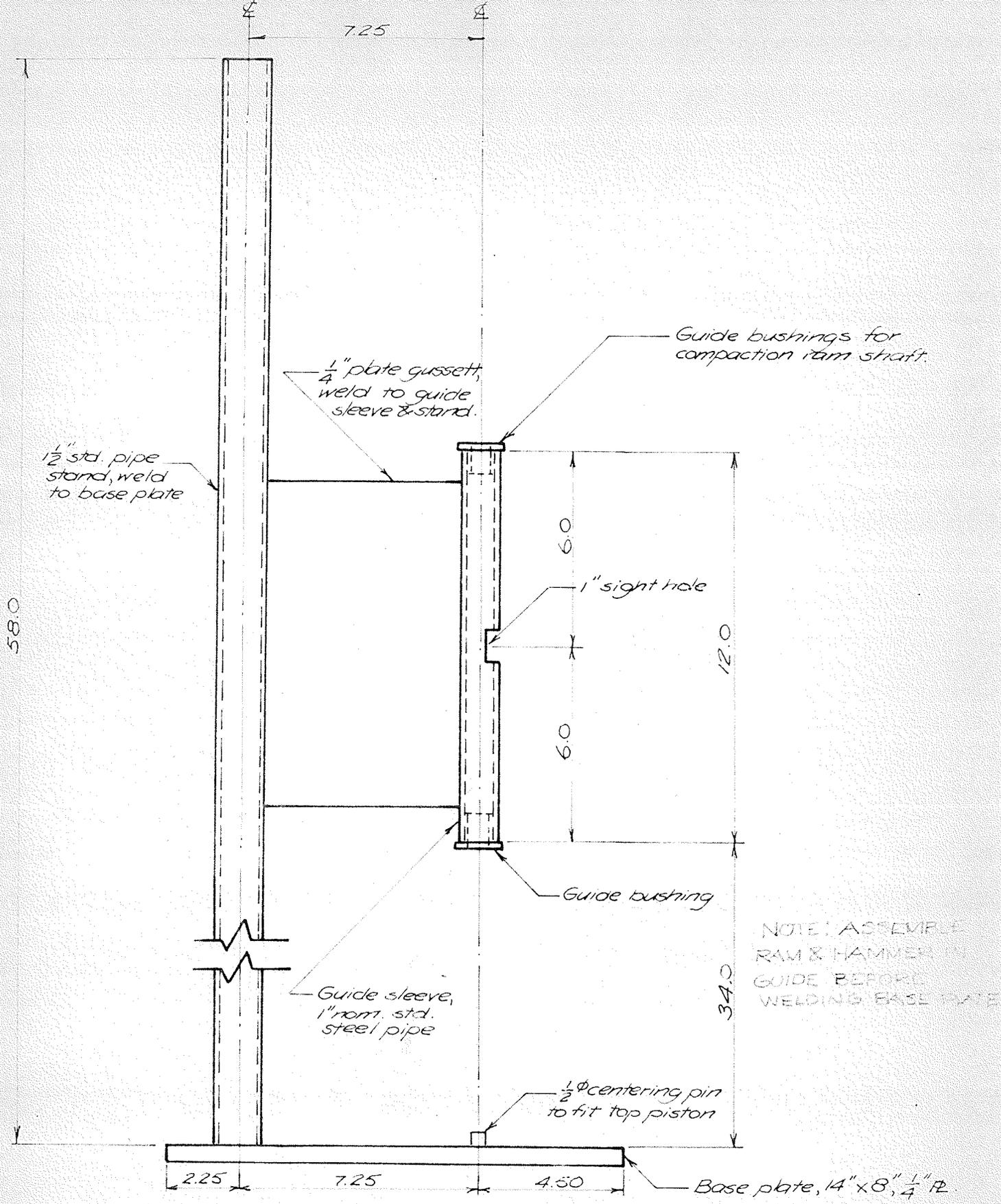
**COMPACTION FRAME - 1 Req'd. (St.1.)**
