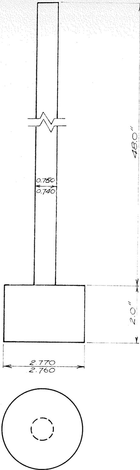
**COMPACTION RAM-1** Req'd. (St'l.)
