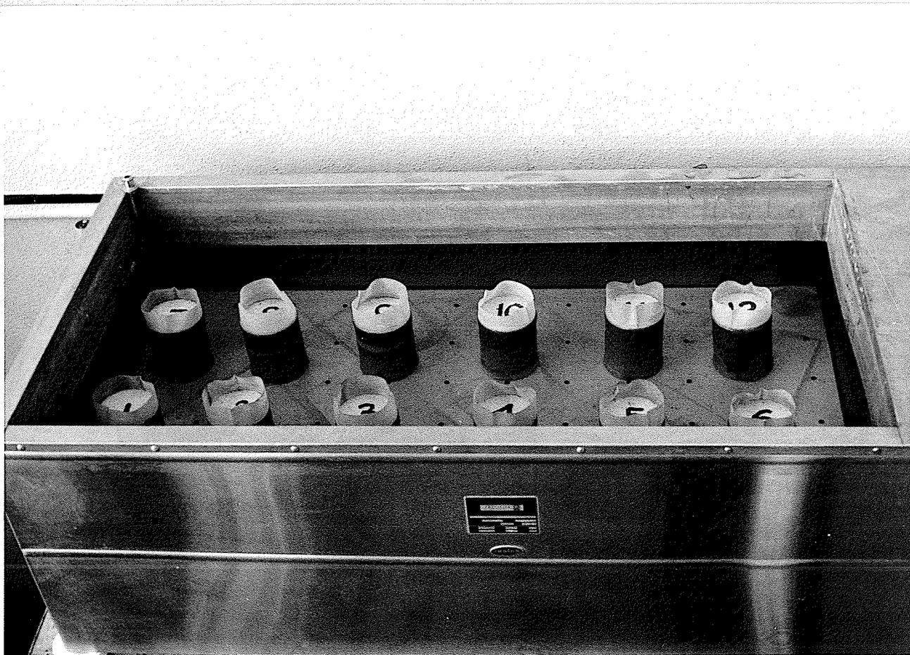
Figure IX Test Specimens in Water Bath
