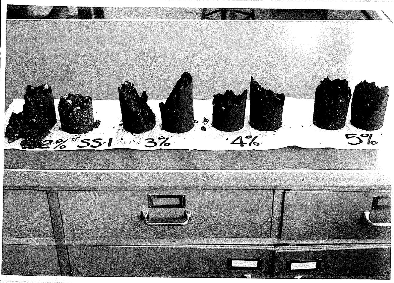
Figure XLII Asphalt-Treated Specimens After Testing
