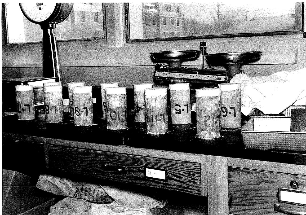
Figure VIII Lime-treated Specimens prepared for Absorption
