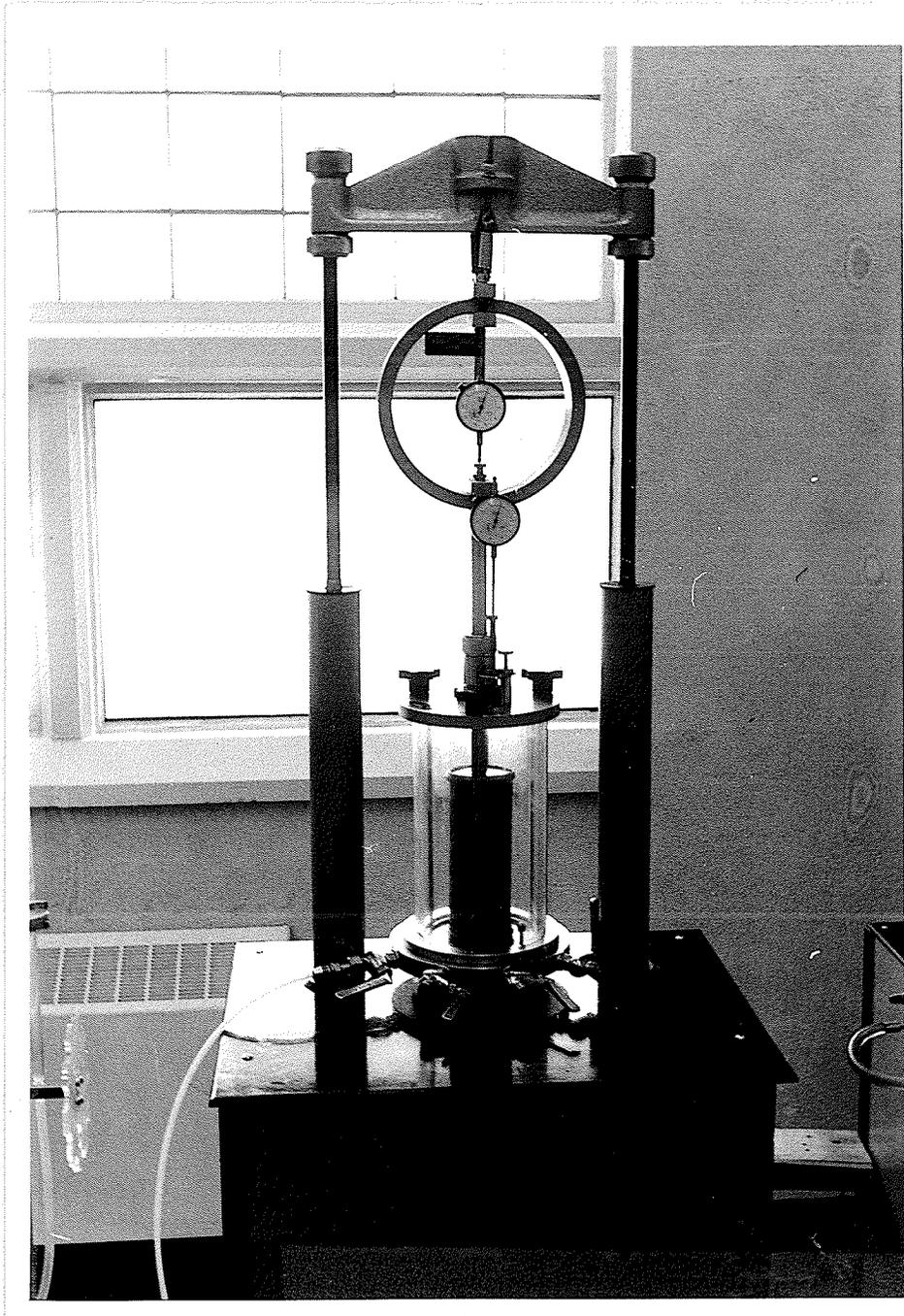
Figure 1 Triaxial Compression Testing Machine
