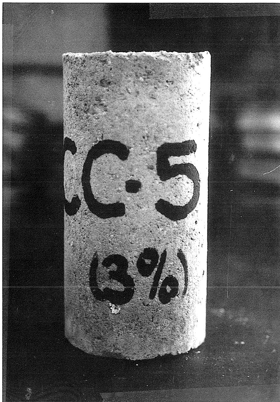
Figure V Calcium Chloride-Treated Specimen After Drying
