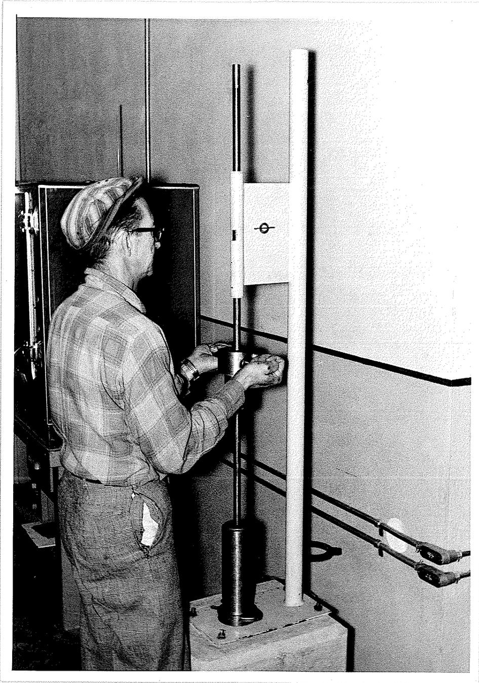
Figure III Moulding Apparatus in Use.
