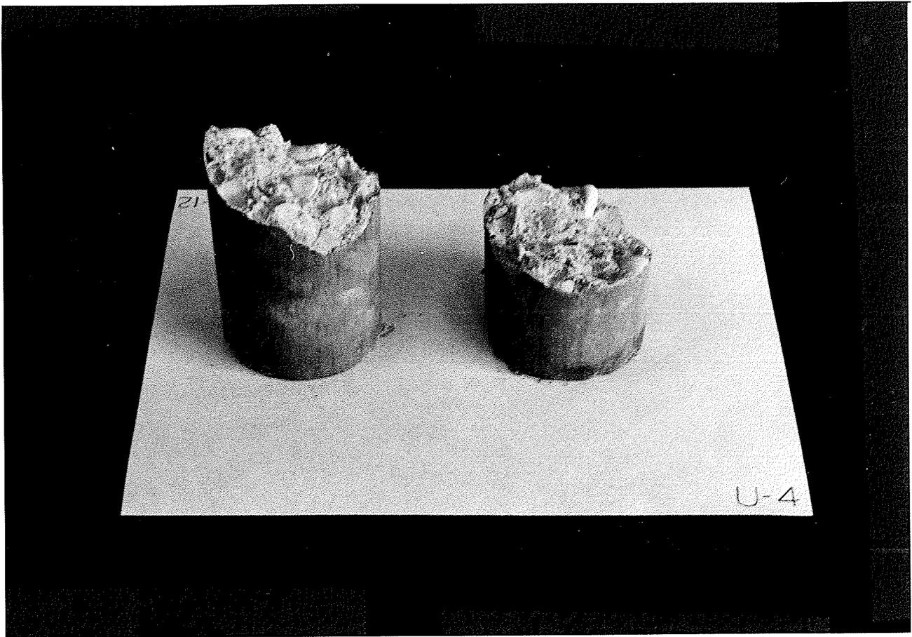
Figure VI Test Specimen after Triaxial Test
