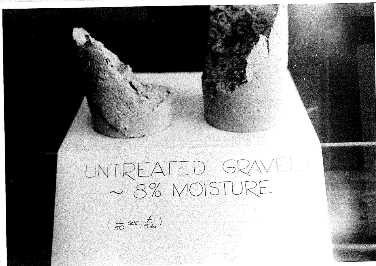
Figure XL Untreated Gravel Specimen After Triaxial Test
