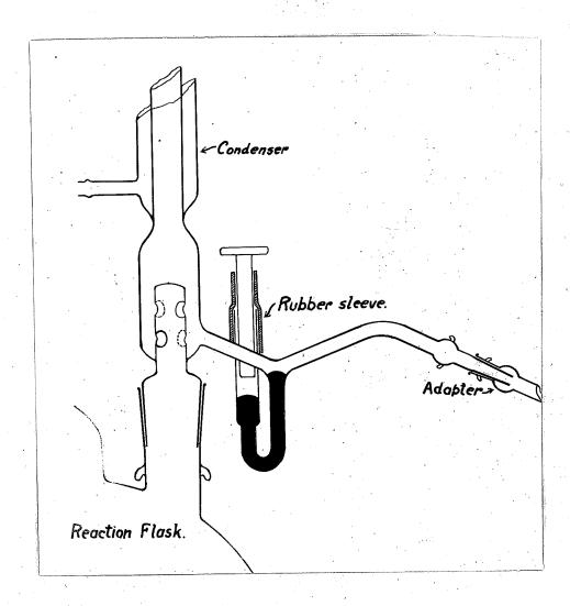
MERCURY VALVE and ADAPTER. (medifications of apparatus illustrated in Fig. 1.)
