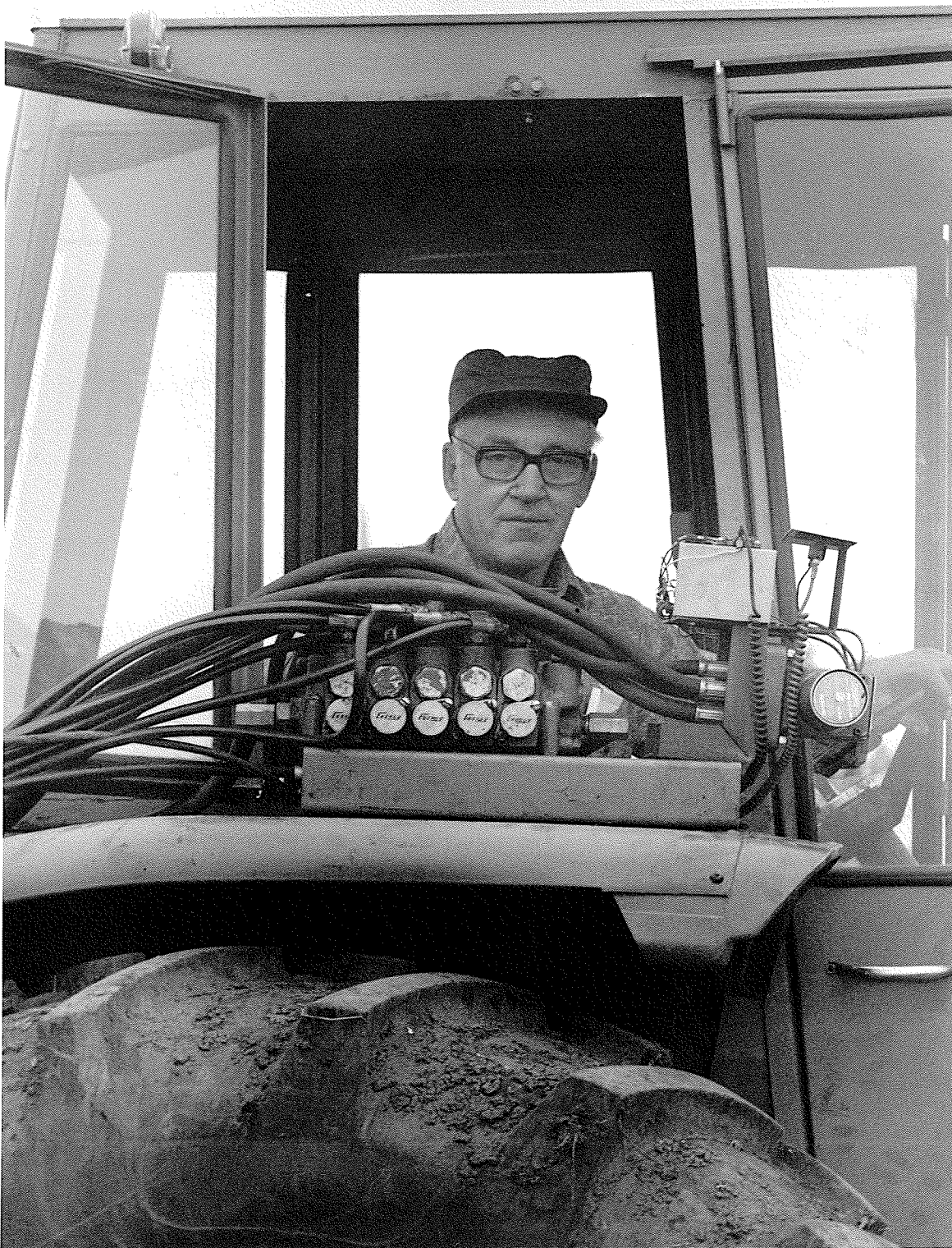
Fig. 3.7 View of Mount for Automatic Control Unit
