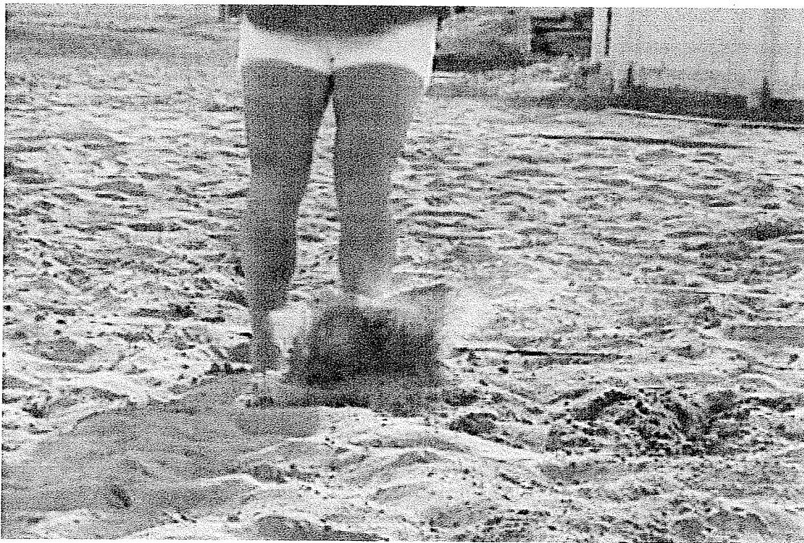
Figure 2.13: Illustration of smaller braking forces resulting from energy absorbed and lost in the softer sand surface. (Front view)
