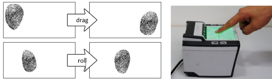
(a) Holz and Baudisch's [11] show fingerprint outline and features move in synchrony when dragging but remain stationary when rolling. (b) RidgePad prototype
