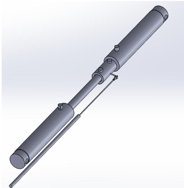
Figure 53: Illustration of Test Cylinder Fully Retracted
