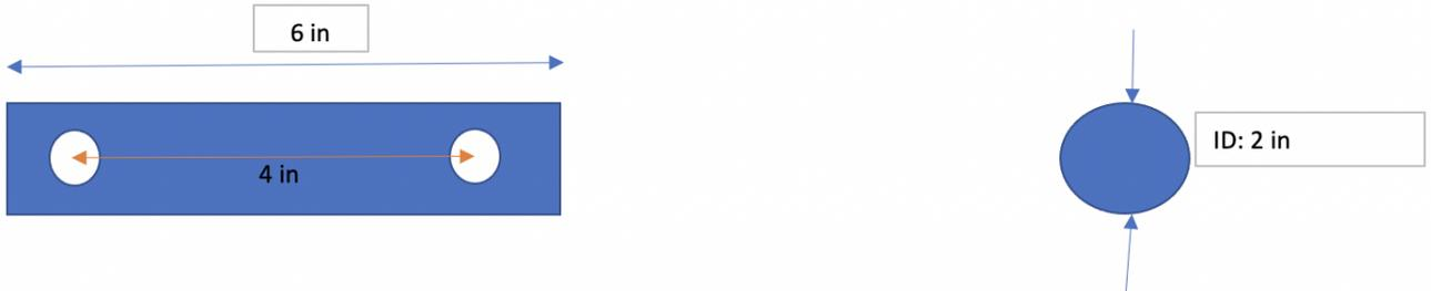
Figure 49: Schematic of Sleeve of Configuration 5
