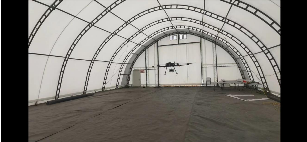
Fig. 3.3. Airborne radar mounted on AAT-1200 during hovering test.
