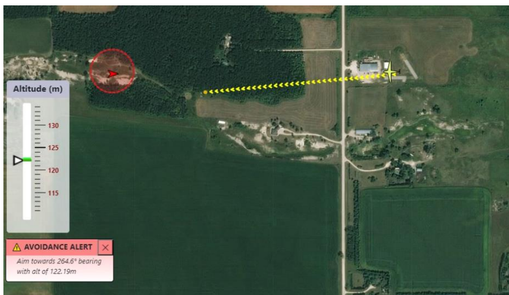
Fig. 4.5. Collision avoidance advisory to an approaching obstacle. The aiming point is between the obstacle and the own aircraft, and it is fixed throughout the flight. See video in DAA_Webpage_Demo.mp4 attached).
