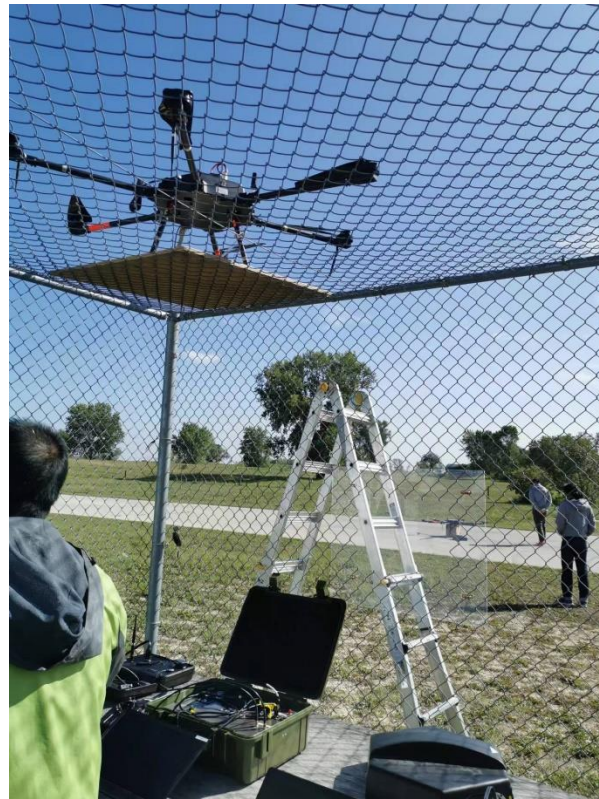
Fig. 3.4. A picture of radar detection flight test setup. The AAT-1200 equipped with radar is placed on top of roof. The airborne radar is expected to detect another UAV which will be taking off on the runway.
