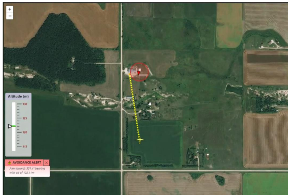
Fig. 4.4. Collision avoidance advisories to a static obstacle.
