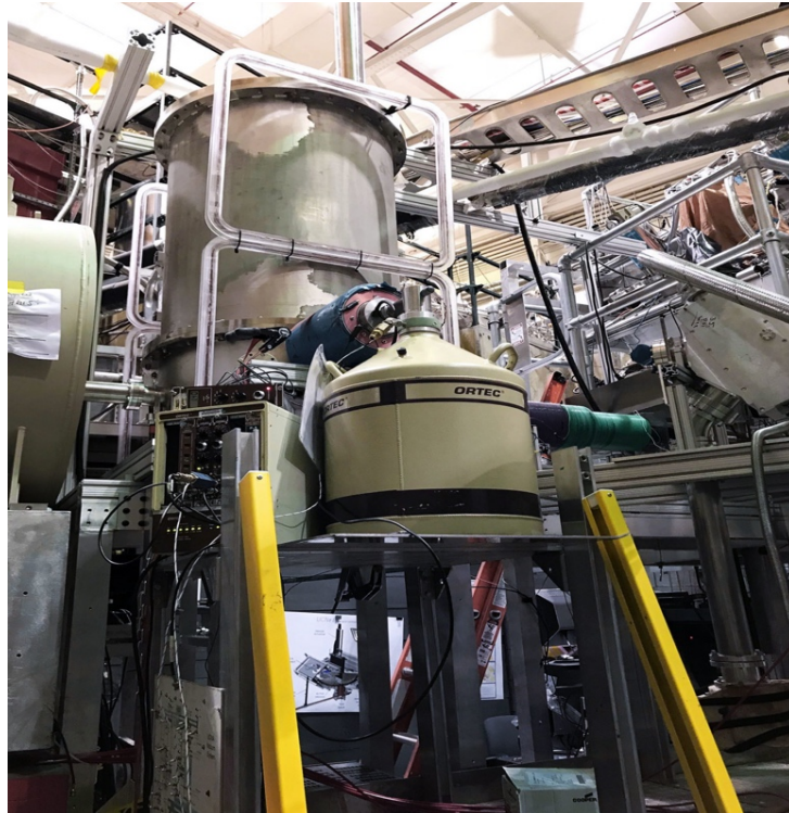
Figure 3. 9 The image shows the Los Alamos National Laboratory's UCNTau experiment measuring the neutron lifespan using the "bottle technique" [20].
