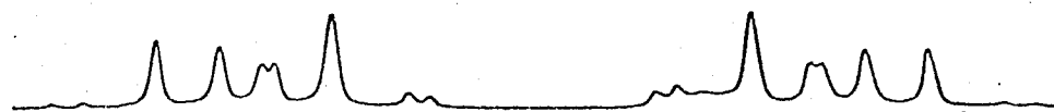
d) 50 cycle scan width of -\text{SiNCOC}_6\text{H}_4\text{CO} region, 10 mole percent solution in deuterated benzene.
