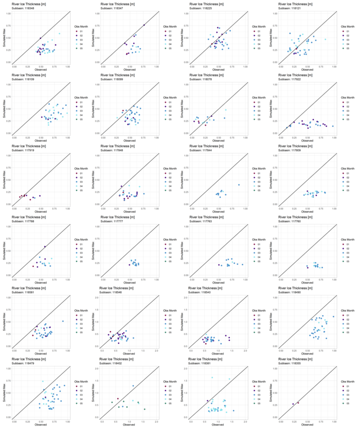
Figure D- 3 Obs vs. Sim annual maximum river ice thickness, colour coded by month of observation [1-24].
