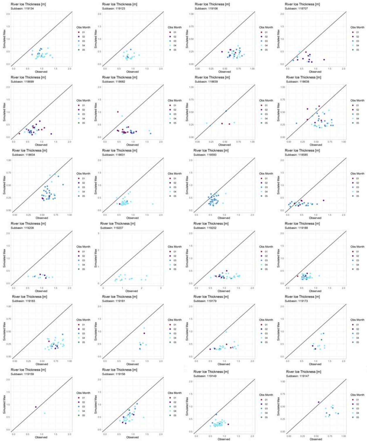
Figure D- 4 Obs vs. Sim annual maximum river ice thickness, colour coded by month of observation [25-48].
