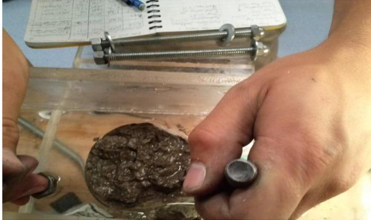
Figure 3.17: Soil sample preparation for EMD test
