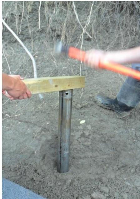
Figure 3.12: Soil sampling procedure using Shelby Tube
