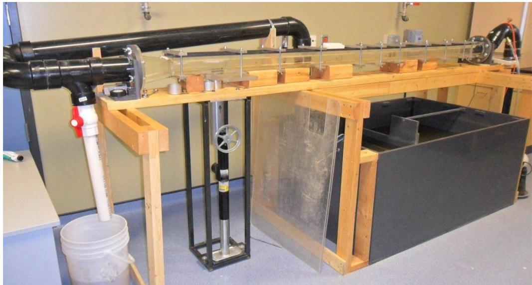
Figure 3.15: Erosion Measurement Device (EMD)
