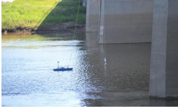
**Figure 3.7: Discharge and velocity measurement from top of the SPB**
