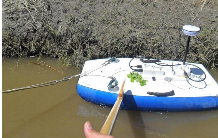
**Figure 3.2: Photograph of the M9 device and hydroboard as close as possible to the bank**
