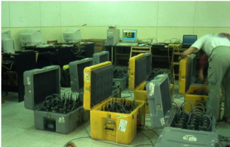
Figure 2.1. TEXAN instrument used for high-density recording in land-based controlled source profiling in southeastern Ireland (Prodehl et al., 2013).
