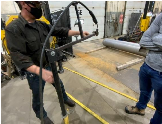
Figure 1: Pipe Spool Welding Torch-Holder
