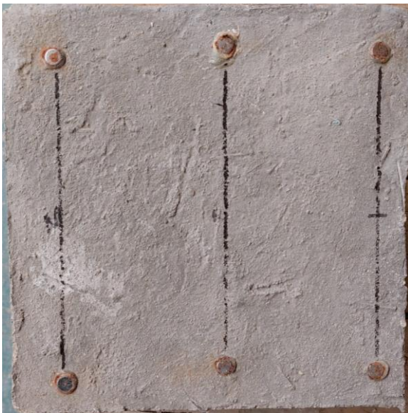
Figure B. 5: Exemplar of restrained shrinkage specimen.
