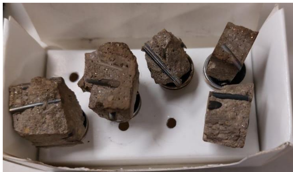
Figure A. 4: Carbon coated specimens for SEM.
