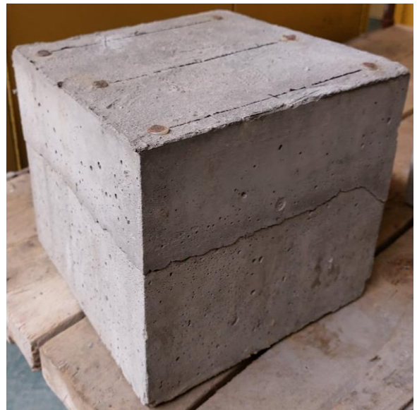
Figure B. 5: Exemplar of restrained shrinkage specimen.
