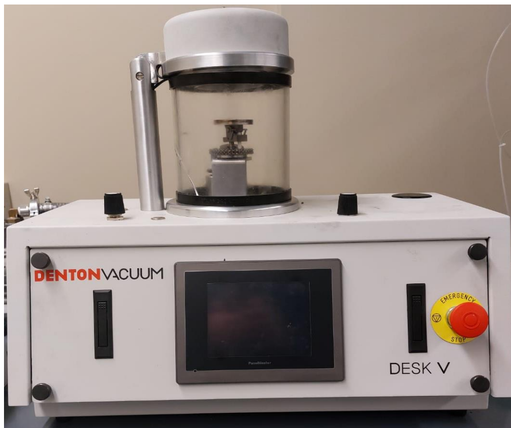
Figure A. 3: Carbon coating machine.
