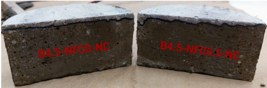
Figure B. 1: RCPT test set-up and exemplar sample after spraying 0.1M silver nitrate.
