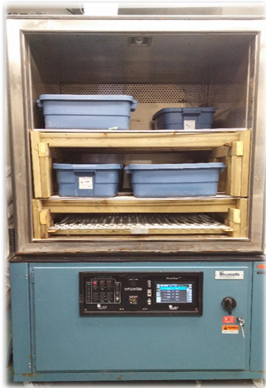
Figure 3. 3: Environmental chamber used for F/T exposure.
