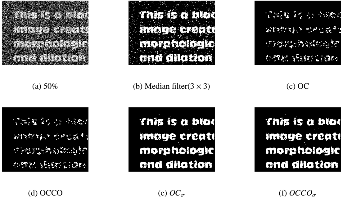
Figure 5.9: Salt and pepper noise removal. (a) Noisy image has a 50% probability of being contaminated with noise, (b) Result of 3 \times 3 Median filter, (c) Open-close sequence, (d) Open-Close-Close-Open sequence (e) Open-close sequence with inclusion degree \sigma = 0.4 (f) Open-Close-Close-Open sequence filtering with \sigma = 0.4 . Structuring element is a 3 square in (c-f).
