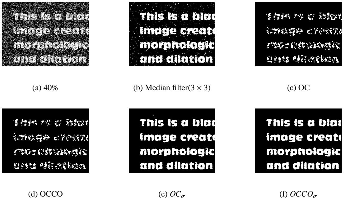
Figure 5.8: Salt and pepper noise removal. (a) Noisy image has a 40% probability of being contaminated with noise, (b) Result of 3 \times 3 Median filter, (c) Open-close sequence, (d) Open-Close-Close-Open sequence (e) Open-close sequence with inclusion degree \sigma = 0.4 (f) Open-Close-Close-Open sequence filtering with \sigma = 0.4 . Structuring element is a 3 square in (c-f).
