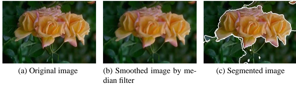
Figure 4.18: Application of median filter on an image(from SIMPLIcity image database [58, 114]) and the segmented result.
