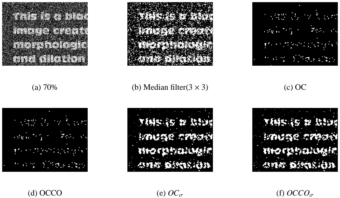
Figure 5.10: Salt and pepper noise removal. (a) Noisy image has a 70% probability of being contaminated with noise, (b) Result of 3 \times 3 Median filter, (c) Open-close sequence, (d) Open-Close-Close-Open sequence (e) Open-close sequence with inclusion degree \sigma = 0.4 (f) Open-Close-Close-Open sequence filtering with \sigma = 0.4 . Structuring element is a 3 square in (c-f).
