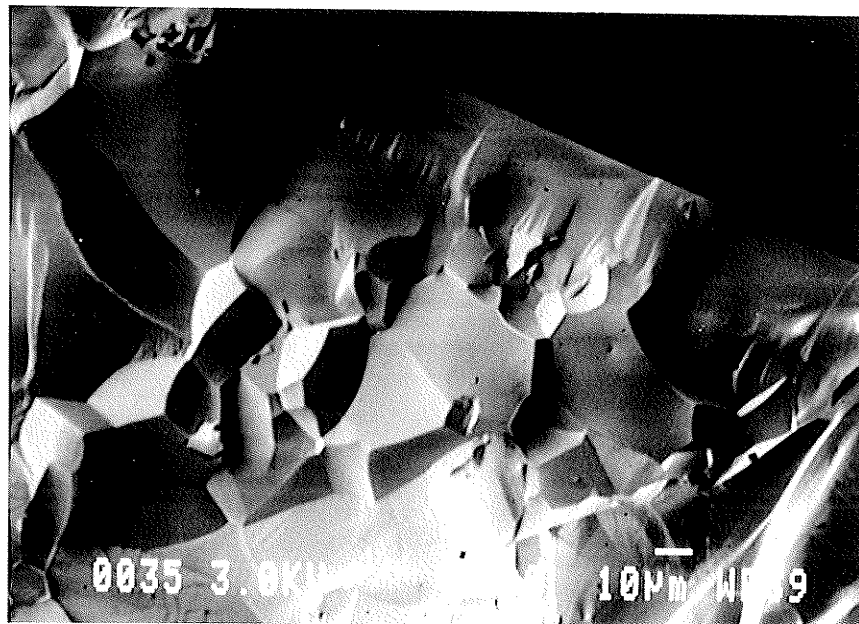
Figure 30: SEM Photograph of the Polycrystalline Bracket Fracture Surface. Note 30 um 'amorphous' layer at bonding surface interface.
