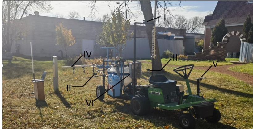
Figure 2. Plot size tractor and the sprayer modified for video recording I-Front Camera, II-Right Camera, III-Left Camera, IV-Nozzle with Solenoid valve, V-Switch to Control Boom, VI-Electric Box
