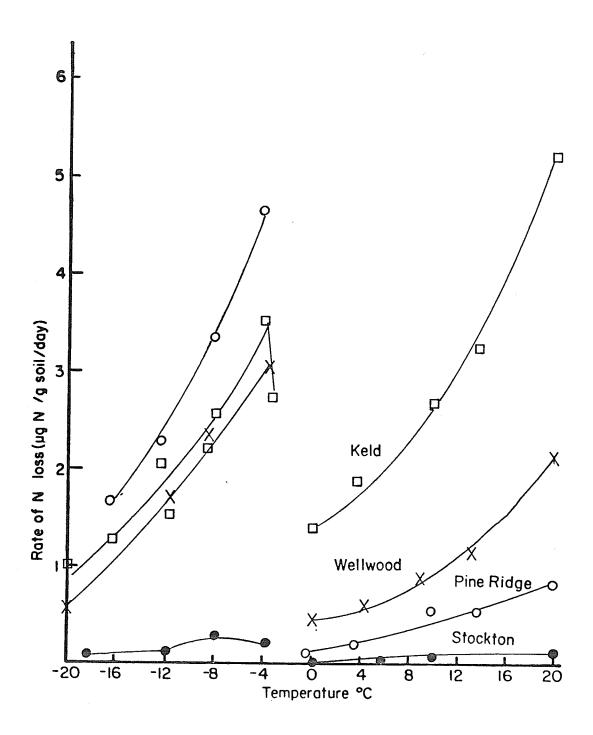
Figure 14: Chemodenitrification of 100 ppm-N nitrite as a function of temperature in Wellwood, Keld, Pine Ridge and Stockton soils.
