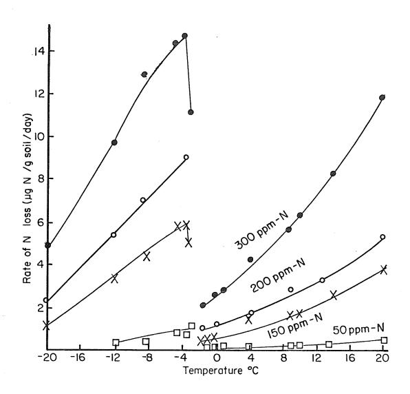
Figure 8: Chemodenitrification rates as a function of temperature in Wellwood soil, 50, 150, 200 and 300 ppm  $NO_2^--N$ .
