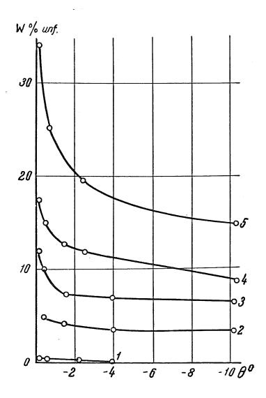
Figure 1: Unfrozen water in typical soils (1) Quartz sand (2) Sandy loam (3) Loam (4) Clay (5) Clay with montmorillonite (Nersesova and Tsytovich, 1963).
