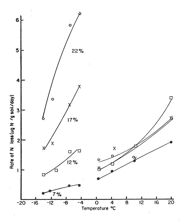
Figure 13: Effect of soil to solution ratio and temperature on denitrification of nitrite in Wellwood soil.
