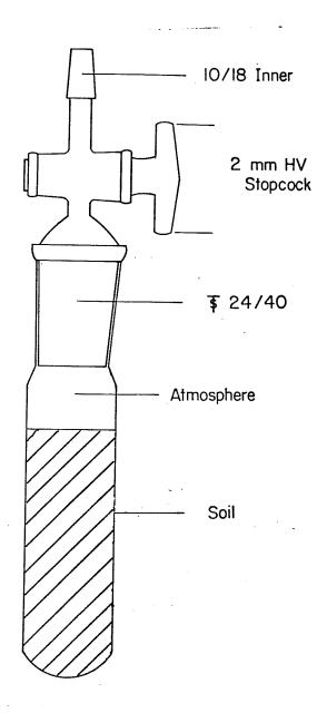
Figure 2: Incubation vessel used in experiments.
