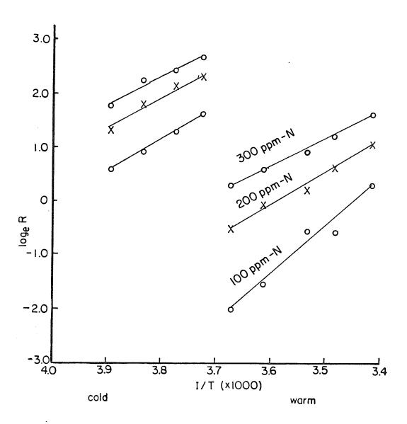
Figure 19: Arrhenius plots of chemodenitrification rates in Pine Ridge soil at concentrations of 100, 200 and 300 ppm  $NO_2^--N$ .
