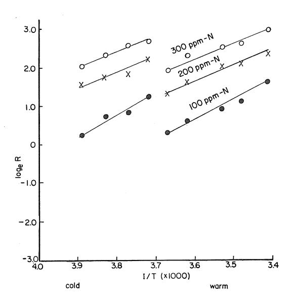
Figure 18: Arrhenius plots of chemodenitrification rates in Keld soil at 100, 200 and 300 ppm  ${\rm NO}_2^-{\rm -N}$  concentrations.
