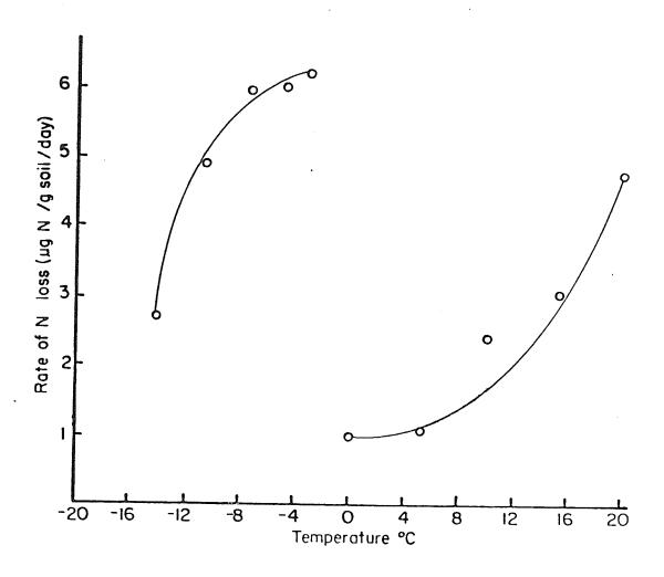
Figure 11: Effect of temperature on the denitrification of 200 ppm-N nitrite in autoclave-sterilized Wellwood soil.
