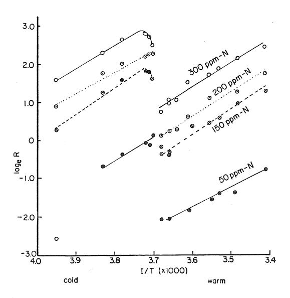
Figure 9: Arrhenius plots of chemodenitrification rates as a function of temperature, 50, 150, 200 and 300 ppm  $^{\rm NO}2^{\rm -N}$ .
