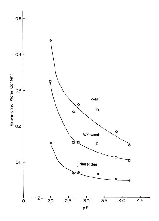
Figure 15: Moisture retention curves of Keld, Wellwood and Pine Ridge soils.
