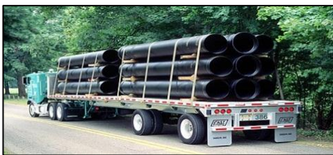
Figure 10: Five axle flat-bed truck with a rear split tandem axle
