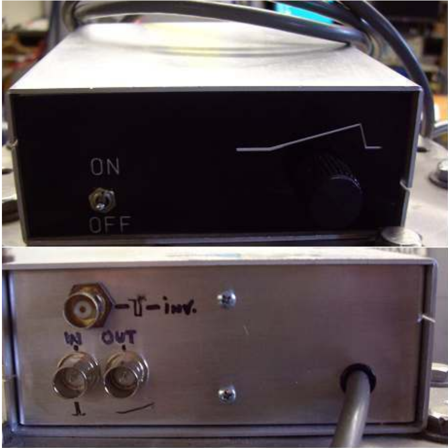
Fig.3-10 New Sawtooth Generator
