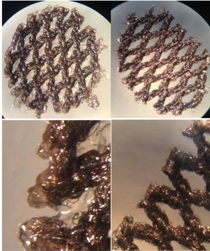
Scheme 3- Observation of Acticoat dressing before and after coating their edges under the microscope. Left pictures are Acticoat-PAM-10 and right pictures are Acticoat sample.
