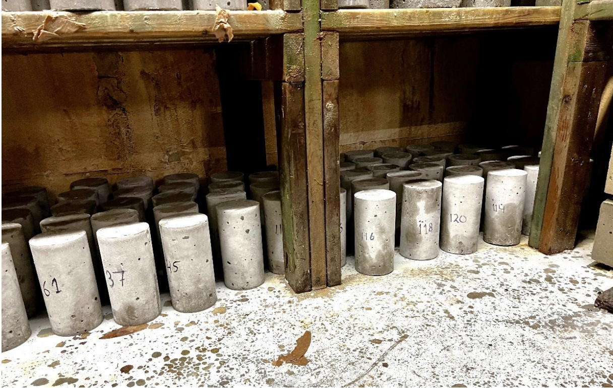
Figure 3-3 Curing of concrete cylinders with labeled ID numbers
