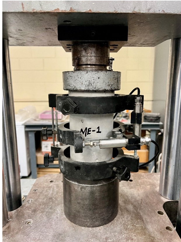
Figure 3-10 Test setup for modulus of elasticity and Poisson's ratio measurement.
