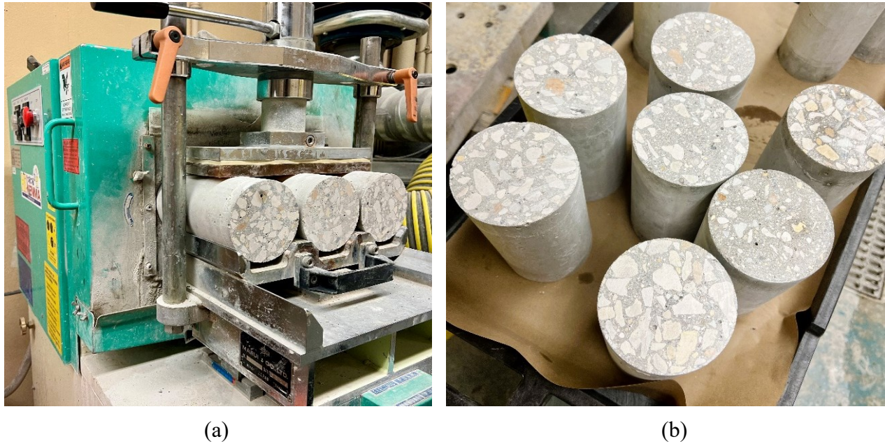
Figure 3-4 Concrete surface preparation. (a) Concrete grinding process in progress using the grinding machine; (b) Surface of concrete cylinders after grinding
