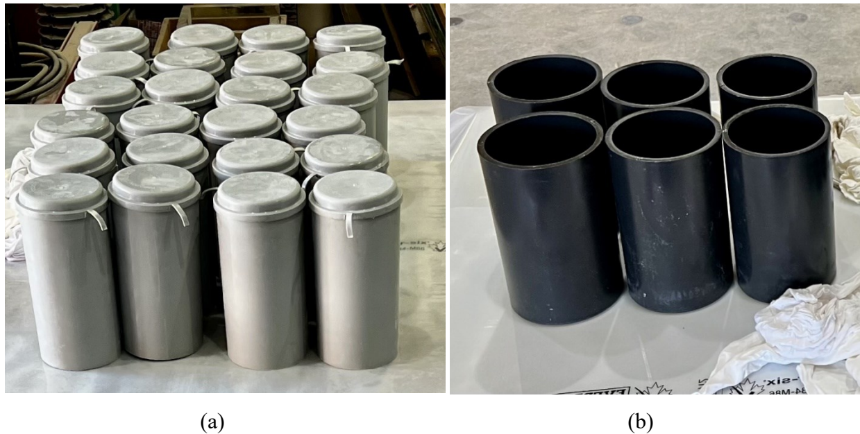
Figure 3-1 Plastic cylinder molds (a) Molds with 3 mm thick walls, equipped with lids; (b) Molds with 6.2 mm thick walls, used without lids
