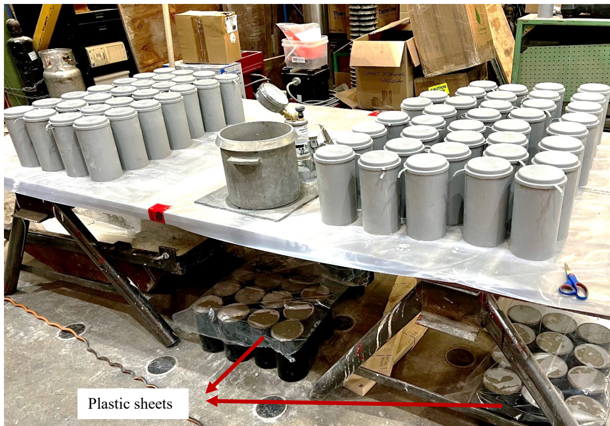
Figure 3-2 Placement of specimens after casting
