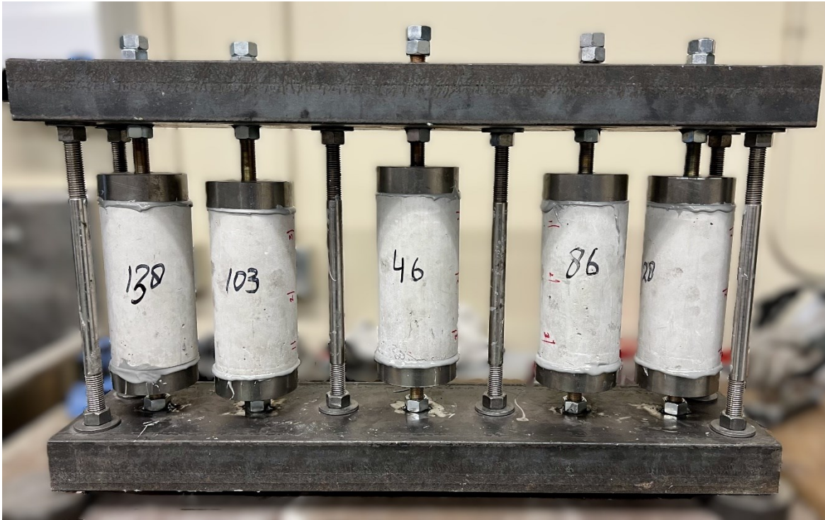
Figure 3-7 Set up for applying epoxy to the steel discs and specimens.
