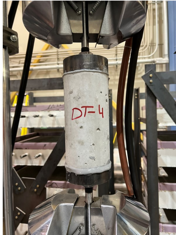
Figure 3-9 Direct tensile testing setup. (a) Schematic of the loading configuration; (b) Actual compressive testing in progress.
