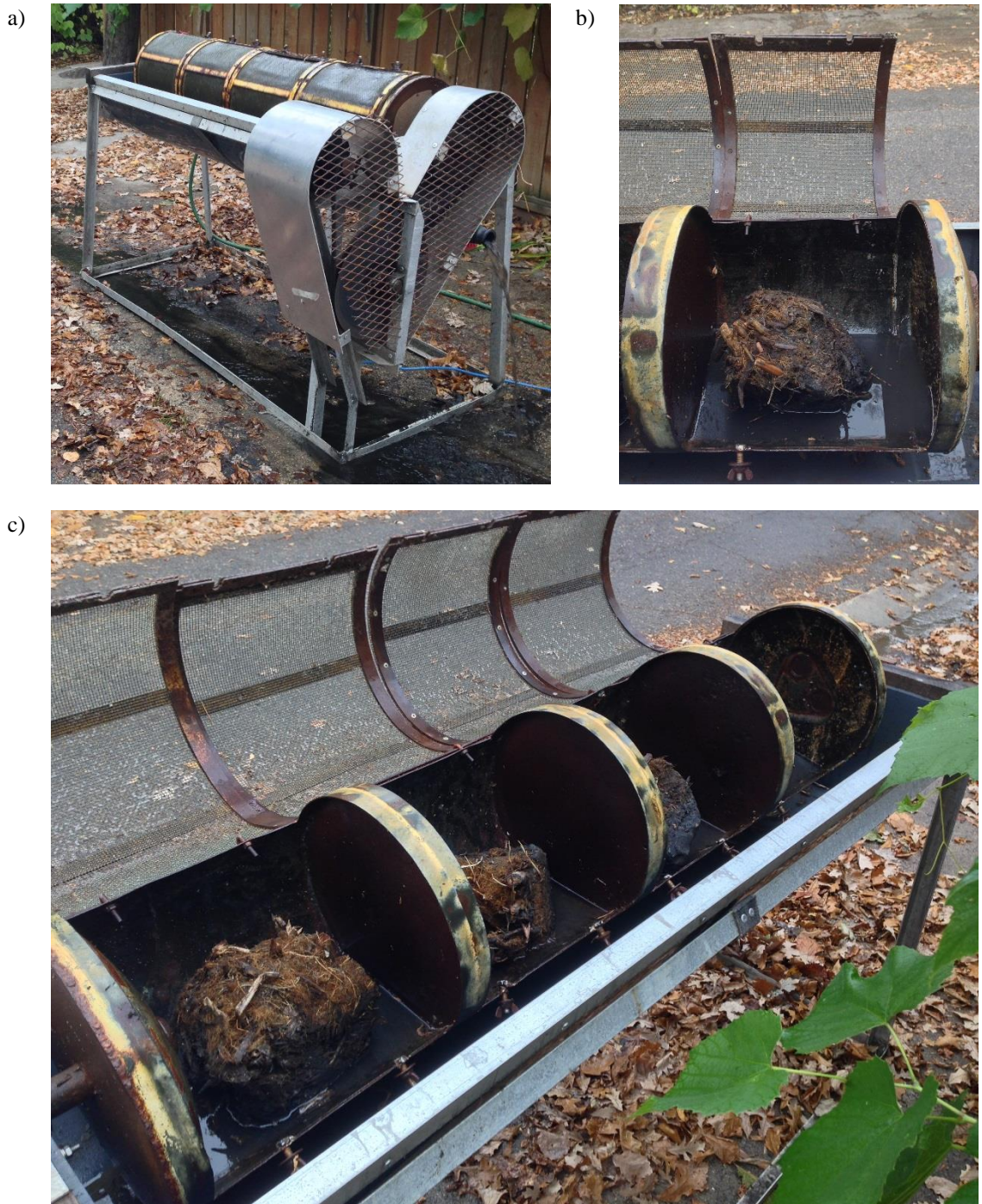
Figure 16. Marsh Ecology Research Program (a) root washer, (b) sample compartment, and (c) rotating compartment drum.
