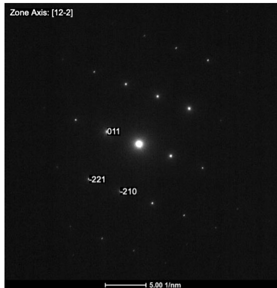
Figure 21: Diffraction pattern of G2 corresponding to [01\bar{1}\bar{2}] zone axis.
