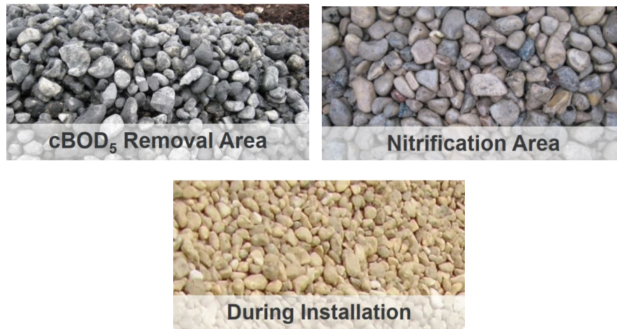
Figure 2.7: Coarse Gravel Biofilm Growth Scenarios - Courtesy of Nexom
