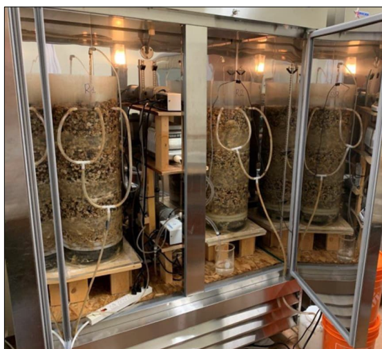
Figure 2.9: Lab-Scale SAGR Photograph - Courtesy of Nexom
