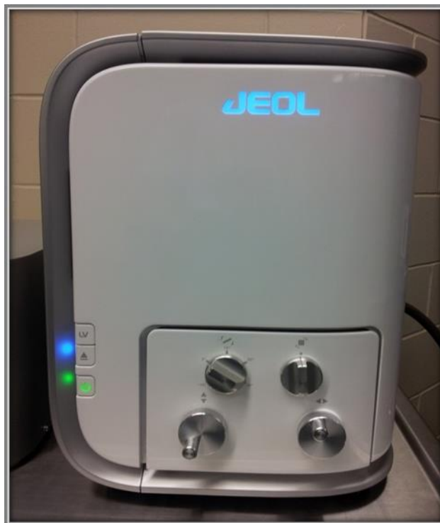
Figure 3. 2: SEM chamber where the fracture specimens were mounted for observation.
