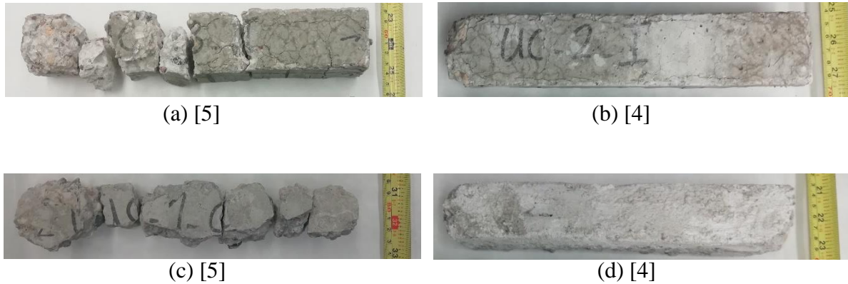
Figure 4. 4. Examples of uncoated concrete specimens: (a) UC- w/b 0.6-full immersion exposure, (b) UC- w/b 0.4-full immersion exposure, (c) UC- w/b 0.6-combined exposure, and (d) UC- w/b=0.4 combined exposure. (Note: numbers between brackets represent the final visual rating).
