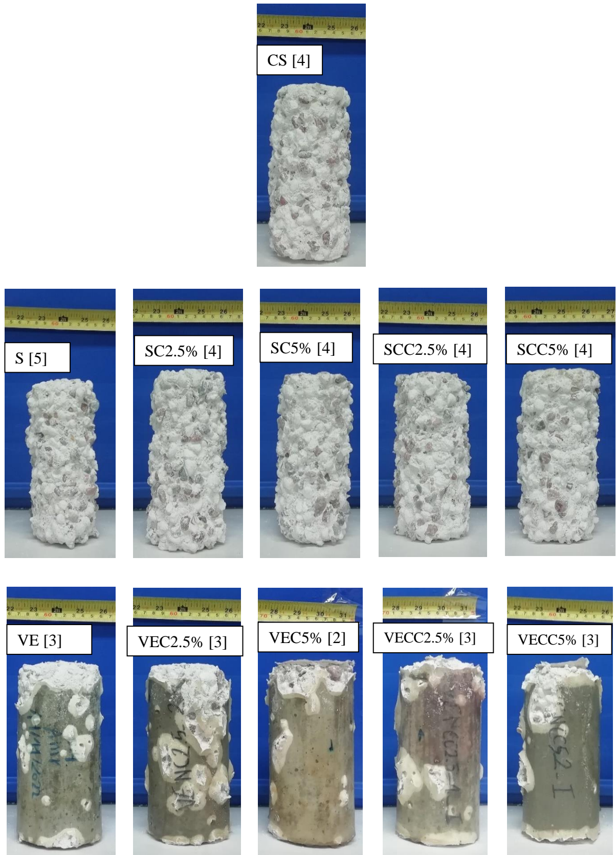
Figure 5. 2. Examples of coated concrete specimens (GU-FA0.4) after 10 weeks in the full immersion exposure. (Note: numbers between brackets represent the final visual rating).
