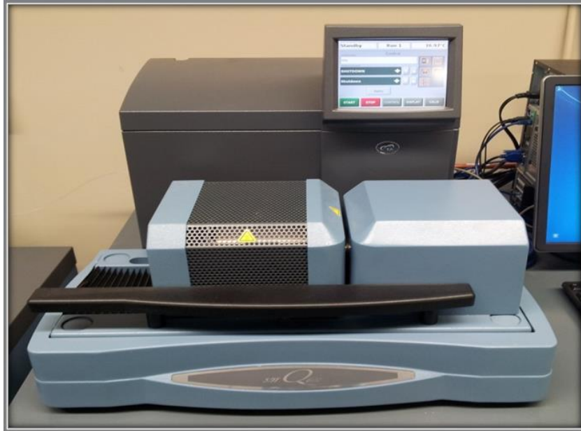
Figure 3. 1: DSC instrument by which the thermal analysis was conducted.
