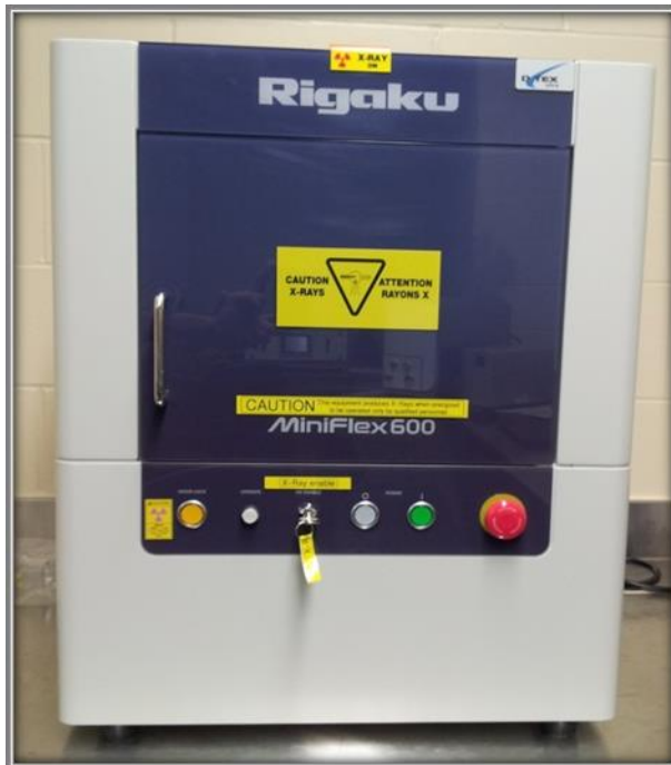
Figure 3. 3: XRD instrument by which the mineralogical analysis was conducted.
