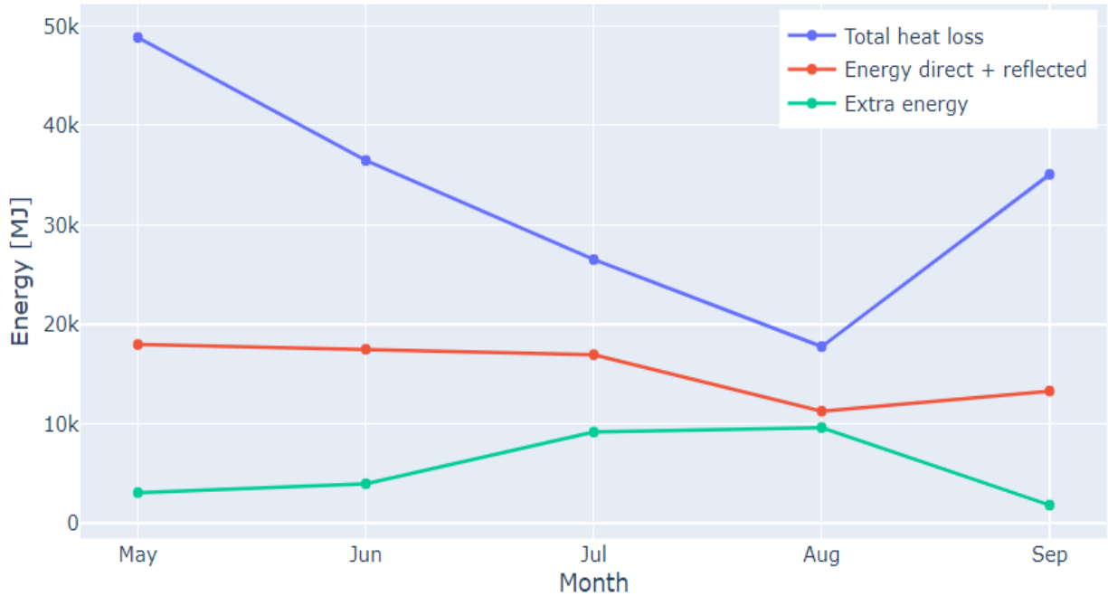
Figure 57: Average monthly heat losses, required energy and extra energy for pool heating
