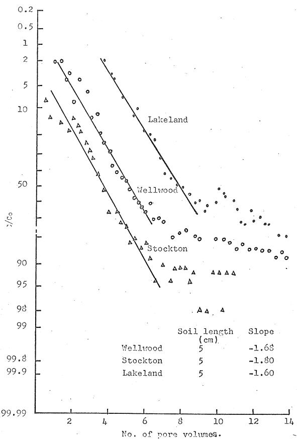
Figure 23. Probability plots of miscible displacement of the three soils.
