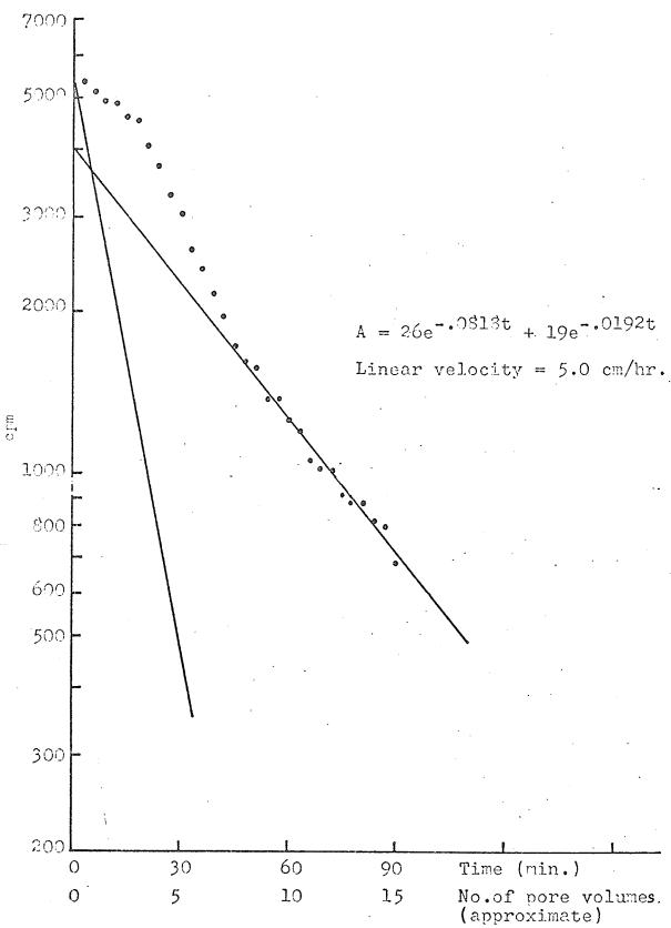
Figure 18. Semi-log plots of the desorption from the Lakeland soil against time.
