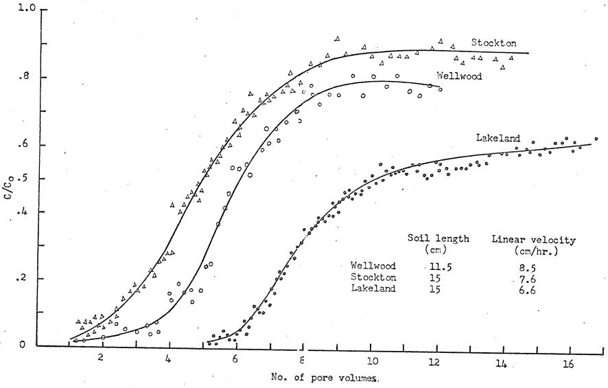
Figure 5. Breakthrough curves for phosphate from the experimental soils.
