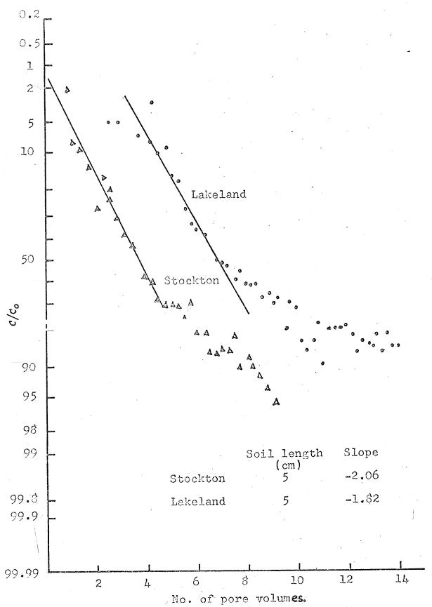
Figure 24. Probability plots of miscible displacement of the two soils.
