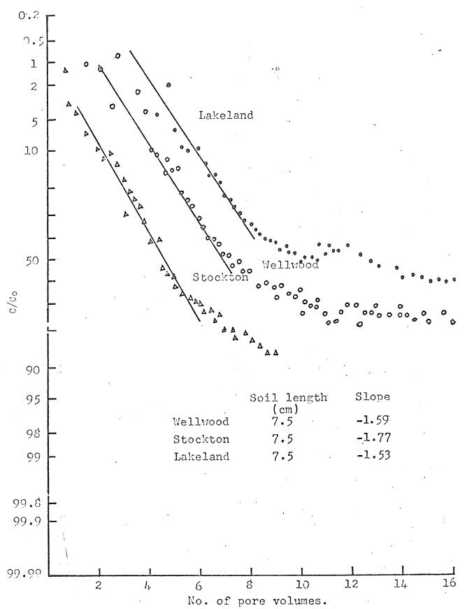
Figure 21. Probability plots of miscible displacement of the three soils.
