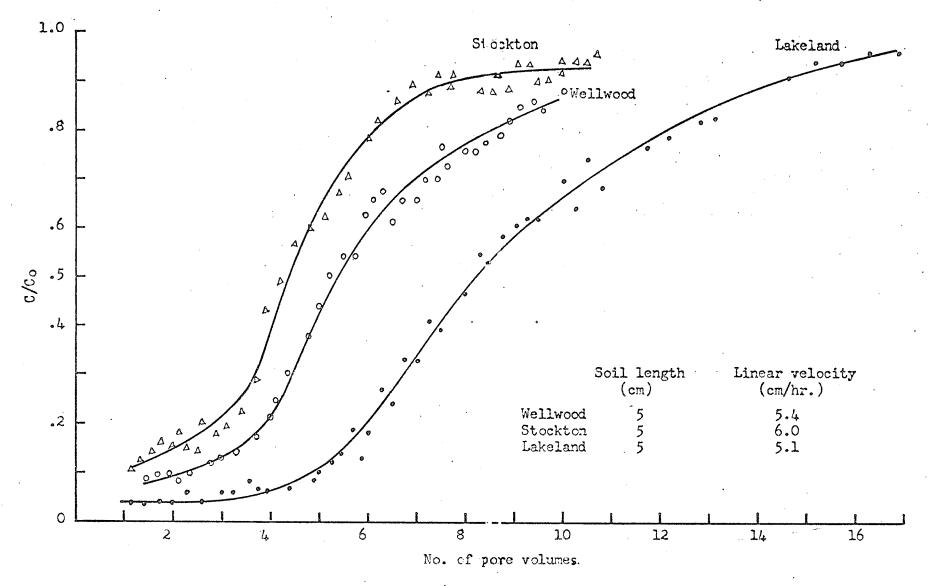
Figure 3. Breakthrough curves for phosphate from the experimental soils.
