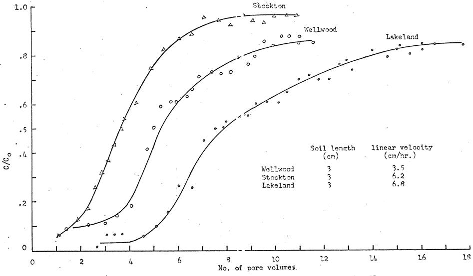
Figure 2. Breakthrough curves for phosphate from the experimental soils.
