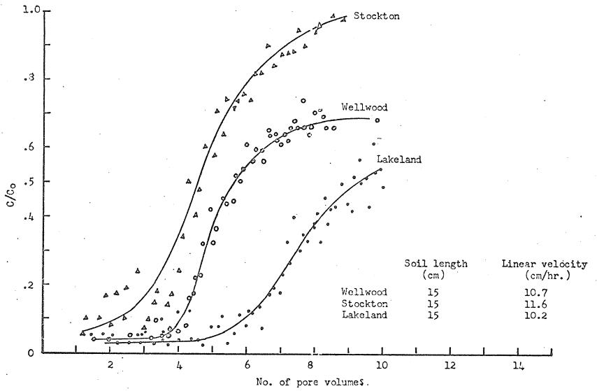
Figure 8. Breakthrough curves for phosphate from the experimental soils.
