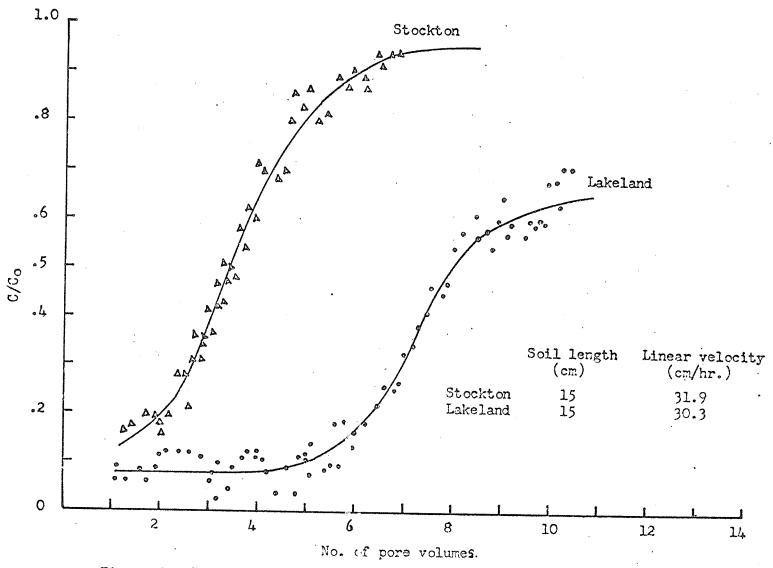
Figure 9. Breakthrough curves for phosphate from the experimental soils.
