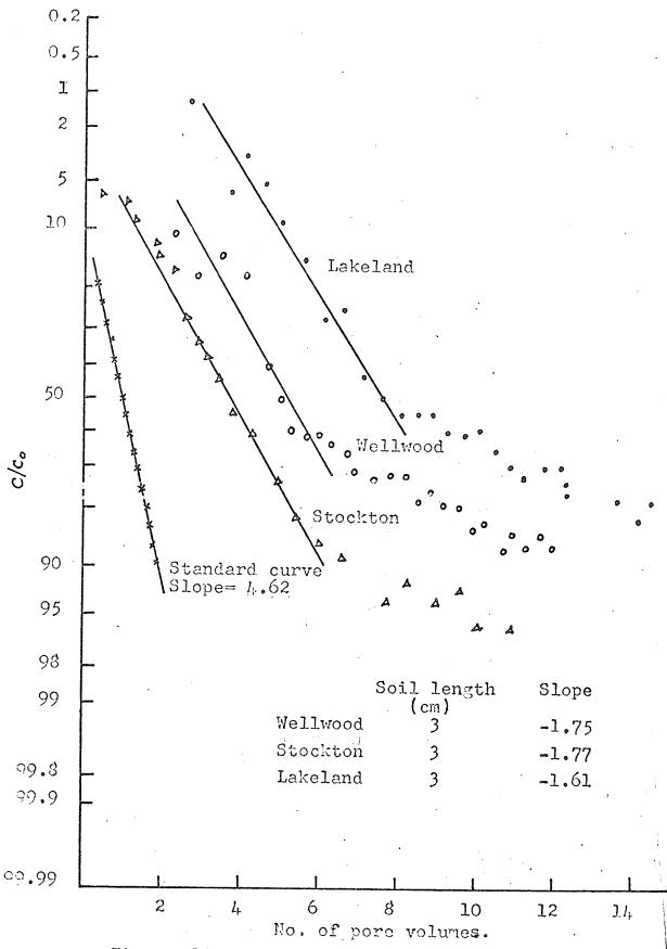
Figure 19. Probability plots of miscible displacement for the three soils.
