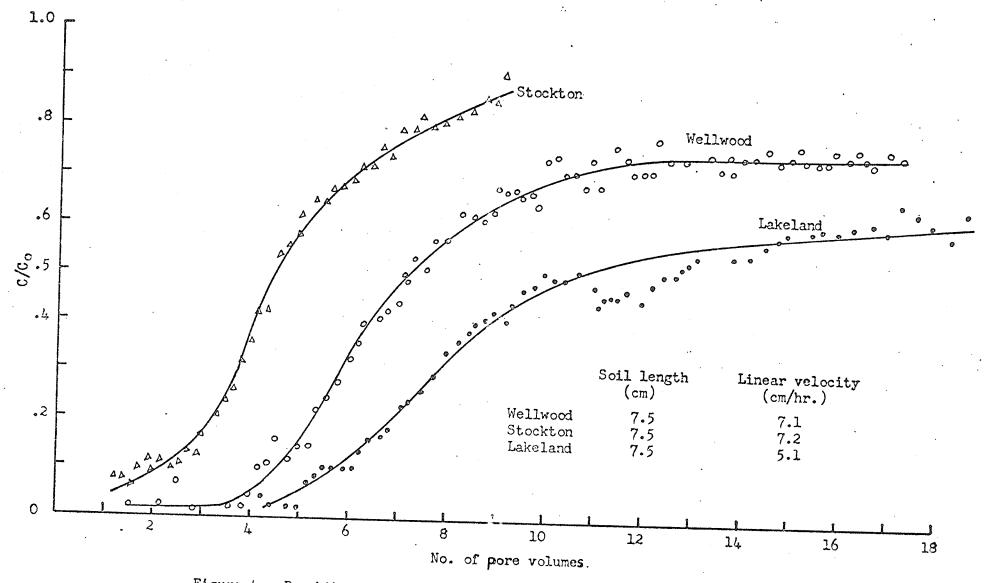
Figure 4. Breakthrough curves for phosphate from the experimental soils.
