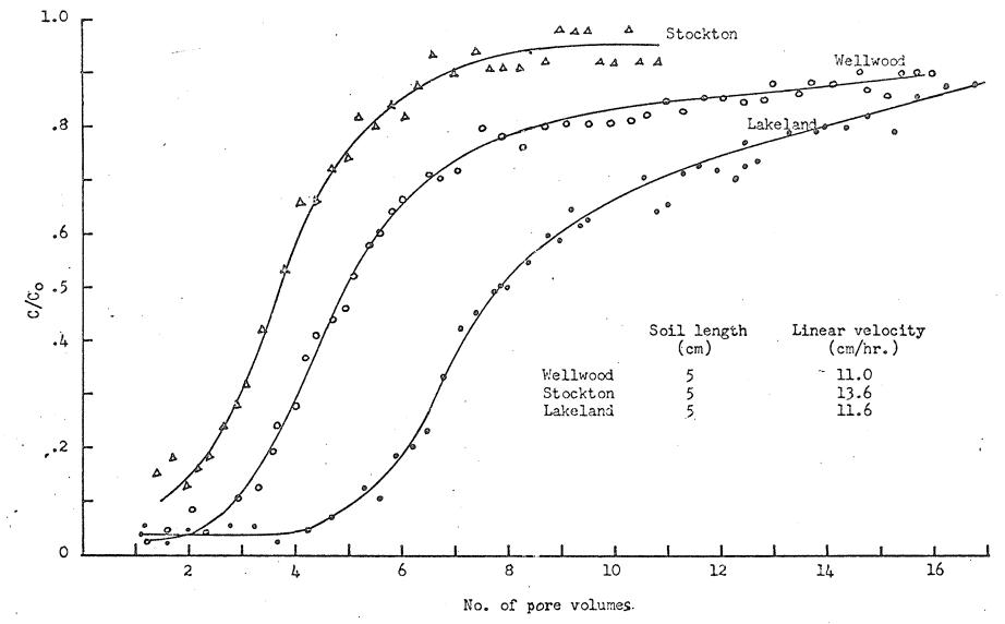
Figure 6. Breakthrough curves for phosphate for the experimental soils.
