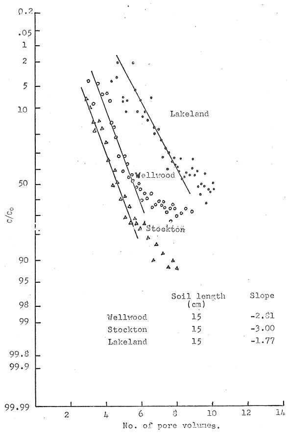
Figure 25. Probability plots of miscible displacement of the three soils.
