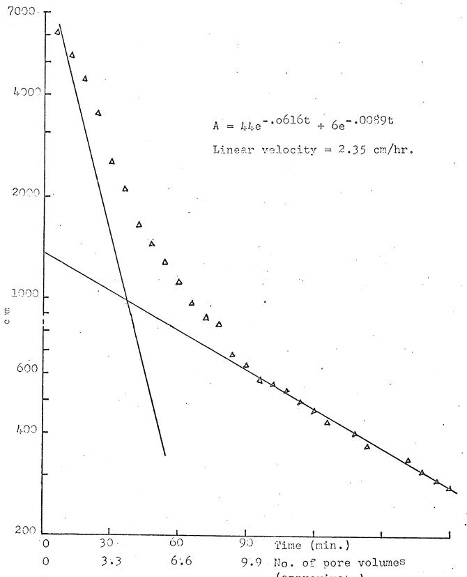
Figure 14. Semi-log plots of the desorption from the Stockton soil against time.
