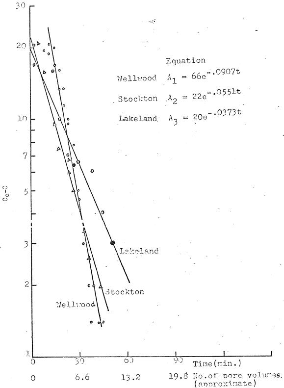
Fig. 11 Semi-log plots of the rate of orthophosphate adsorption by the three soils with the fast rate.
