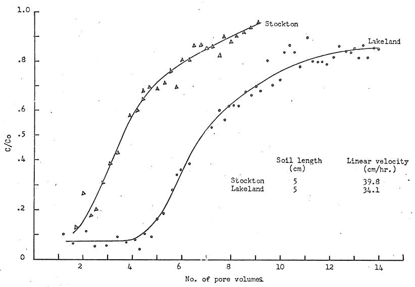
Figure 7. Breakthrough curves for phosphate from the experimental soils.
