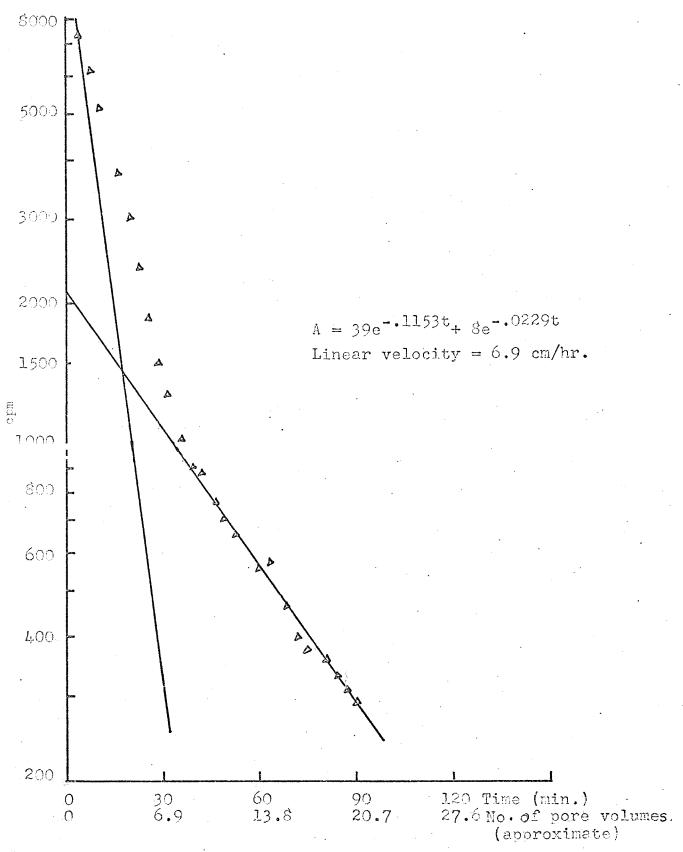
Figure 17. Semi-log plots of the desorption from the Stockton soil against time.
