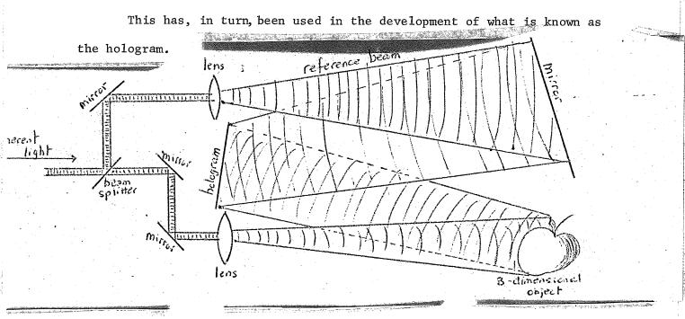
Coherent light from a laser is split by a semitransparent mirror, half of the beam being called the reference beam which is reflected by means of mirrors onto a photographic plate (transparency); the other half of the
