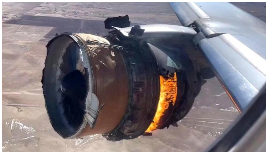
Figure 3. An example of Aviation Gas Turbine Failure
