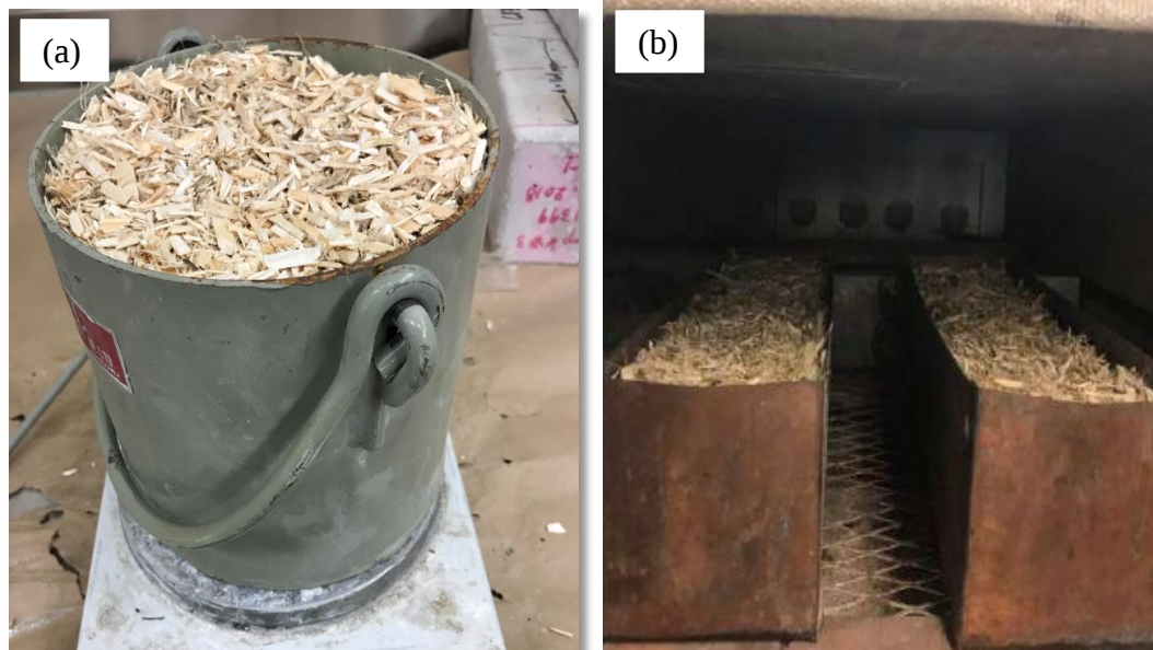
Figure 1: (a) Measurement of bulk density and (b) oven drying of hemp hurd
