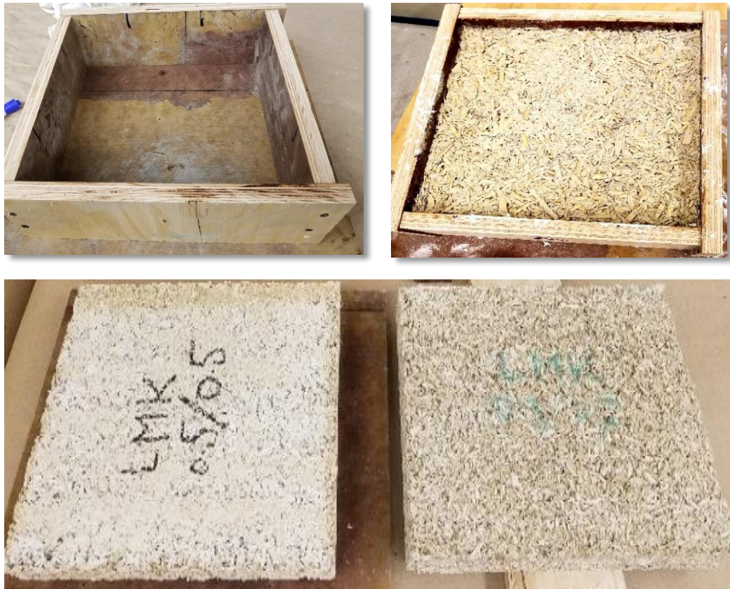
Figure 6: Test samples for thermal conductivity measurements
