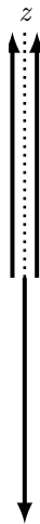
Figure 3.11: When the magnetic field strength H = \frac{zJ}{2} , two spins on the triangle completely align with the field while one remains anti-aligned in a collinear state
