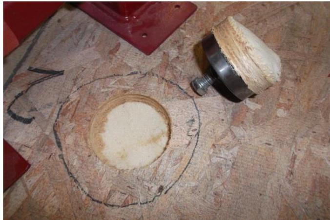
(b) Failure within the foam-core
