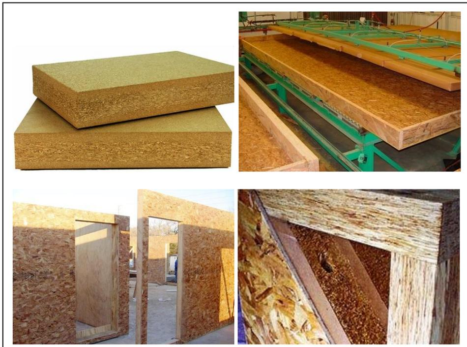
Figure 2-5: SIPs made of compressed wheat straw, Timber Strand sub-frame, Exposure 1 OSB, (7/16 in. - no urea formaldehyde added) and, non-toxic adhesives (Agriboard Industries , 2010)
