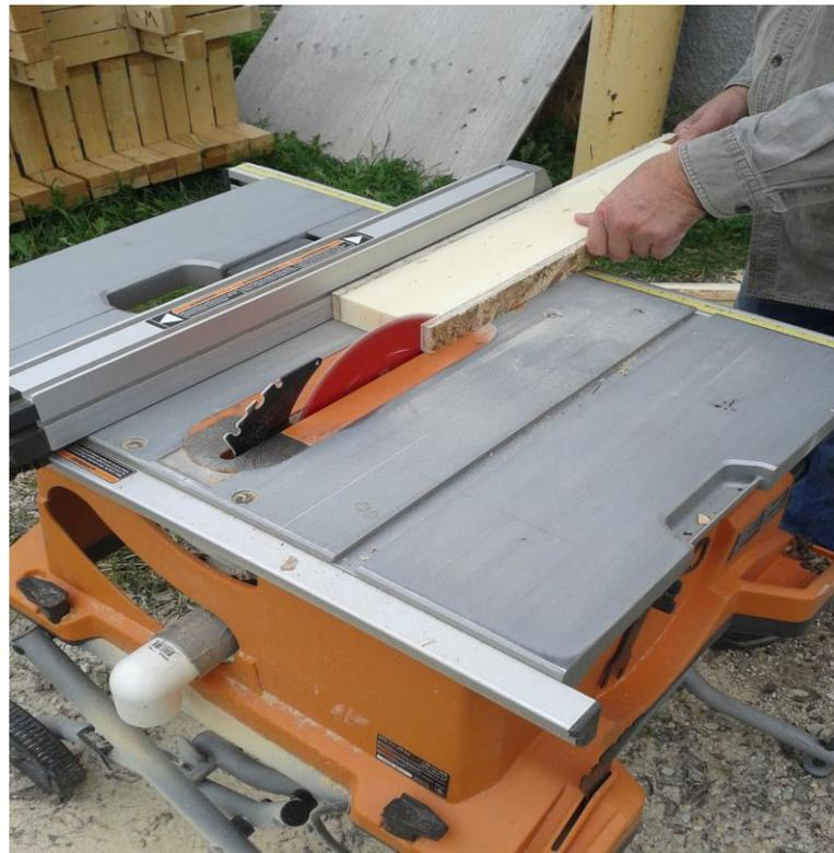
Figure 7-2: Separating OSB face-sheets from the PUR foam-core
