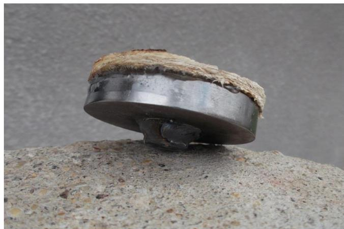
(c) Failure within the OSB face-sheet
