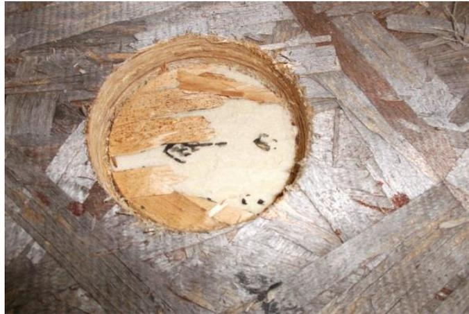
(a) Partially de-bond failure
