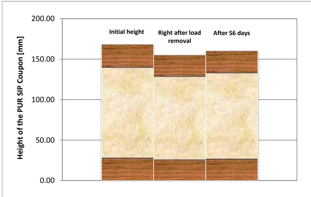
**Figure 5-3: Relaxation and rebound behaviour of 165mm (6.5 in.) thick PUR SIP coupons under compressive load**
