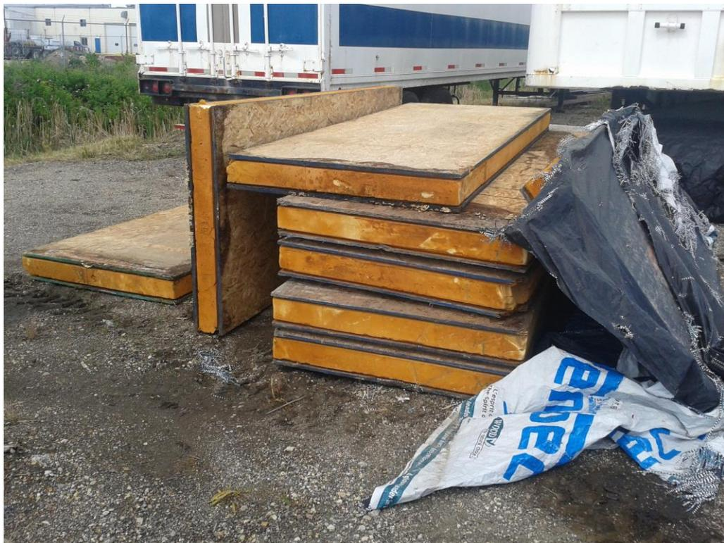
**Figure 6-3: PUR SIPs stored in a storage yard with minimum weather protection for more than four years**
