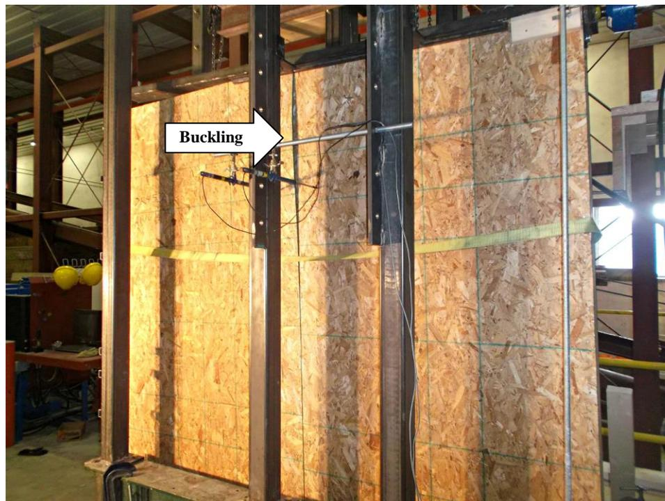
Figure 4-17: Racking test on dis-bonded in progress. Buckling of the dis-bonded area of the left panel can be seen
