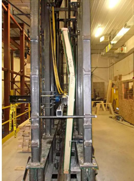
**Figure 4-6: A failed disbonded panel subjected to transverse load**
