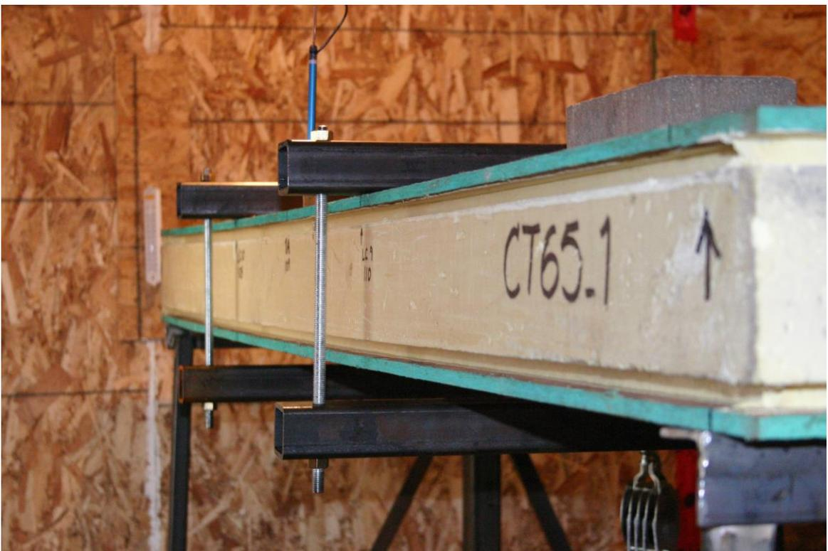
Figure 5-8: Flexural creep test of PUR SIP in progress
