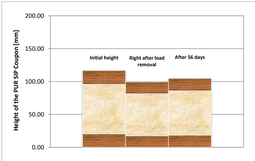
**Figure 5-4: Relaxation and rebound behaviour of 114mm (4.5 in.) thick PUR SIP coupons under compressive load**
