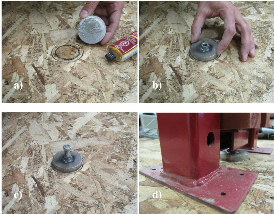
**Figure 6-5: Steps in pull off test preparation**
