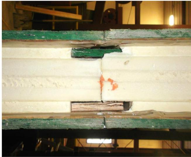
**Figure 4-3: Connection details of two 1220x2440 mm (4x8 ft.) panels joined together for racking test purposes. OSB splines, construction adhesive, expandable spray PUR foam and nails used to join the panels together**
