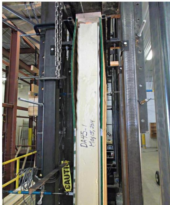
**Figure 4-5: Dis-bonded panel under direct eccentric axial load. Buckling occurred only at the disbonded area of the panel at the time of failure**
