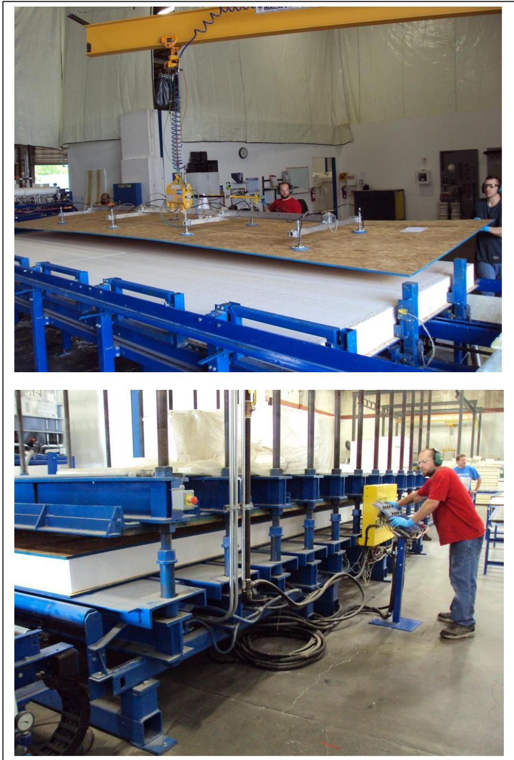
**Figure 1-3: Assembly line of EPS core SIPs (Photo courtesy of Premier SIPs by Insulfoam, United States, 2012)**
