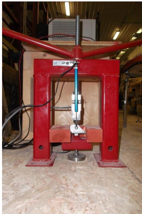
**Figure 6-2: Hand-made pull-off tester used conduct pull off tests on PUR SIPs**
