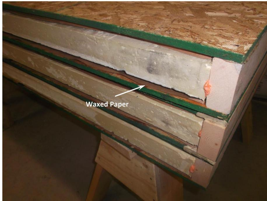
**Figure 4-2: Partially bond-less PUR SIPs ready for test. Waxed paper used between the OSB face-sheets and the PUR foam to avoid bond between the two materials**
