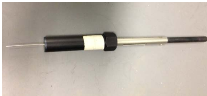
Figure 9. HS-SPME 100 \mu\text{m} polydimethylsiloxane (PDMS) SPME fibre.
