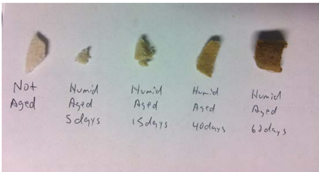
Figure 49. Accelerated humidity aged wool over a period of 62 days at 80°C, 80% relative humidity.
