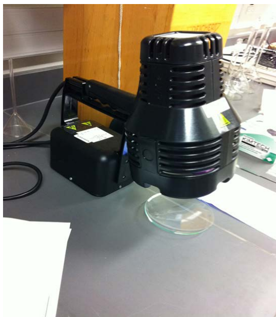
Figure 37. The aging process using UV light from Black-ray B100AP (100W bulb) high intensity UV lamp (365nm long wave UV source).
