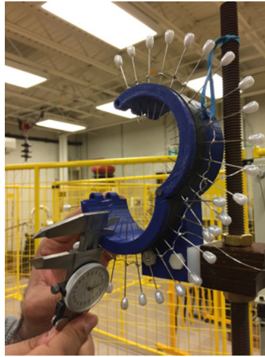
Fig. 4.9: Adjustment of needles using a caliper for investigating the effects of the needle-to-surface separation distance.
