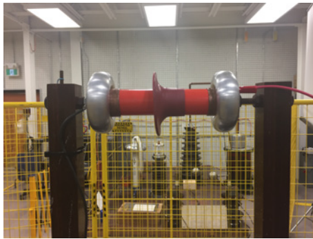
(a) FRP sample with the shed in middle middle
