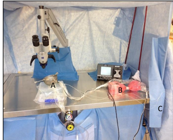
Figure 2: Drilling set-up. (A) Bowl-type holder (B) Transmitter for Acsension TrakSTAR system (C) Cables for sensors
