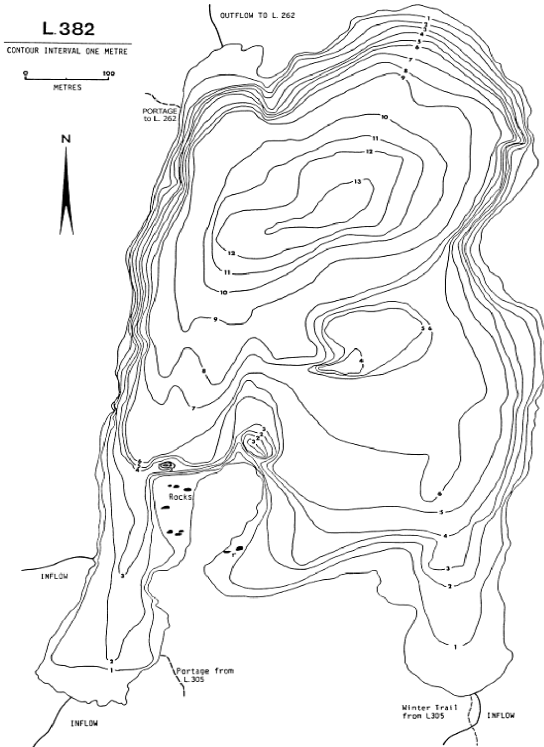
Figure 3.1: Bathymetric map of Lake 382 (ELA Data Retriever provided by Susan Kasian, Department of Fisheries and Oceans, Winnipeg, June 2009). Numbers represent depths in metres
