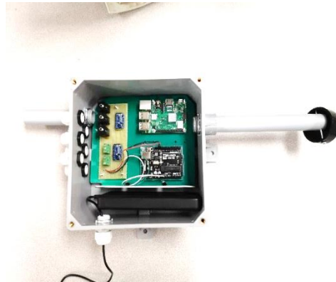
Fig. 3.9 Raspberry-Pi & Arduino integrated system
