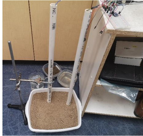
Fig. 3.7 Laboratory data collection with SEN0193 sensors.
