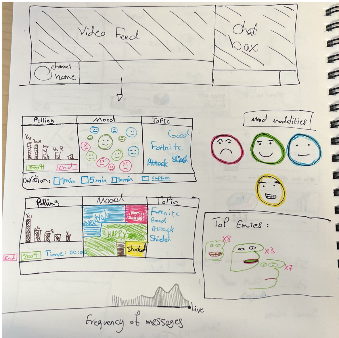
Figure K.2: These sketches depict various data representations for the Polling, Emotes, and Word Cloud features. Originally, the Emotes feature was named 'Mood features,' and we explored different data representations, including emojis, Twitch emotes, and sentiment keywords. Similarly, the Word Cloud feature was initially conceived as both a list and a scatterplot of words. Additionally, we experimented with different placements for the slider features, originally considering the use of Start/Stop buttons and preset time duration buttons.
