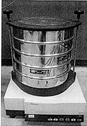
Fig. 4.5. Retsch sieve shaker: screens and collecting pan used for sizing.
