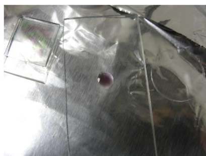
Figure C5.7 Sample preparation by placing a few drops of LC1 doped with 5 wt% of AuNP3 on a microscope slide at Iso-N temperature with no NP settling and turbidity.
