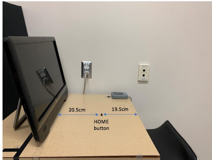
Figure 1. Set up and dimensions of the apparatus. The home button is located 19.5cm away from the edge of the table. Targets displayed on the screen are located 14.75cm to the left and right of the center of the screen.
