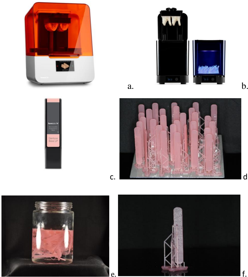
Figure 8. a. Form 3B printer, b. Form Wash and Form Cure, c. Denture Base resin, d. Printed samples on the print plate, e. Samples in glycerin jar for post curing, f. Cured sample before support was removed
