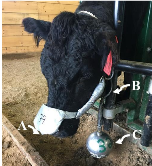
Figure 3. Halter and vacuum ball fitted to each intake heifer to measure CH 4 output while grazing over a 24-hr period; A = intake tube where CH 4 , SF 6 , and CO 2 emissions are captured from the nose and mouth, B = tubing that transfers the exhaled from the heifer's nose and mouth to the evacuated collection ball, C = stainless steel vacuum ball that collects exhaled air.
