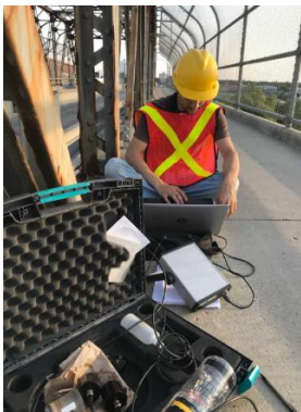
a) UPV test at site
