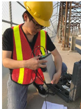
a) UPV test at site
