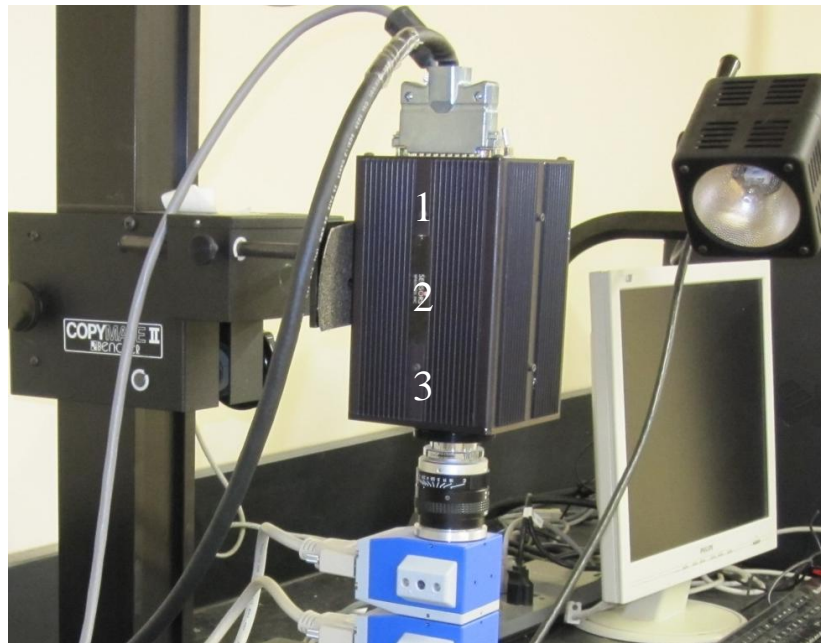
Figure 3.2 Thermocouple locations on the camera
