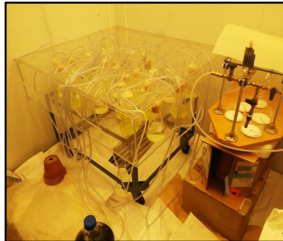
Figure 6. The experimental set-up for duckweed (A) and algae (B) grown in a walk-in chamber with aeration and flow control manifold (photo by Kozlova T.A).
